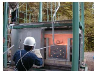
Fig.4 The charcoal is taken out from the furnace.
