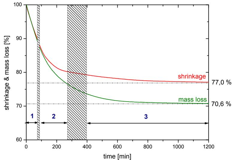
**Figure 3.** Bourry diagram for feedstock PF MCMB 6-G with a water content of 30 wt.%. Mass loss and shrinkage were measured simultaneously, the opening gap between the two lines denotes the development of porosity.
