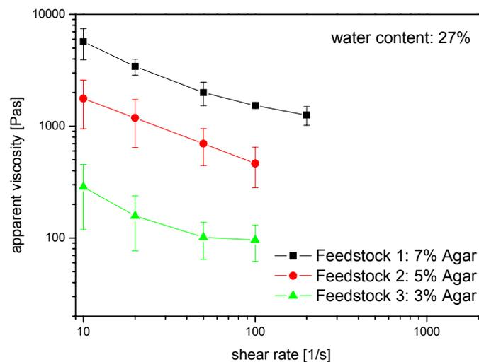
**Figure 2.** Dependency of the rheological properties on the agar content. Lowering the agar content decreases viscosity, however at the cost of less process stability, as indicated by the growing error bars.
