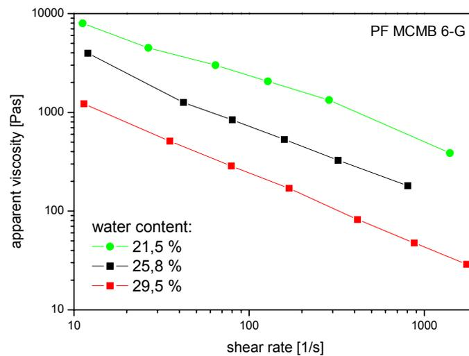
**Figure 1.** Dependency of the rheological properties on the water content. As expected, lowering the water content leads to a distinct increase in viscosity. All samples were prepared in the same way and had an agar content of 6 wt.%.
