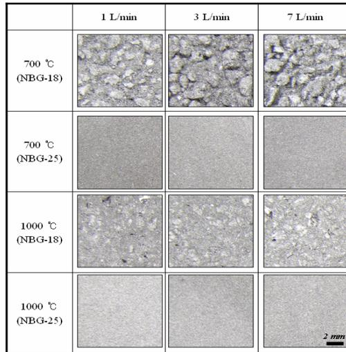
Figure 2. Oxidized surfaces of NBG-18 and NBG-25 (Oxidation Temp.: 700 and 1,100 °C, Flow rate: 1, 2, and 7 L/min).
