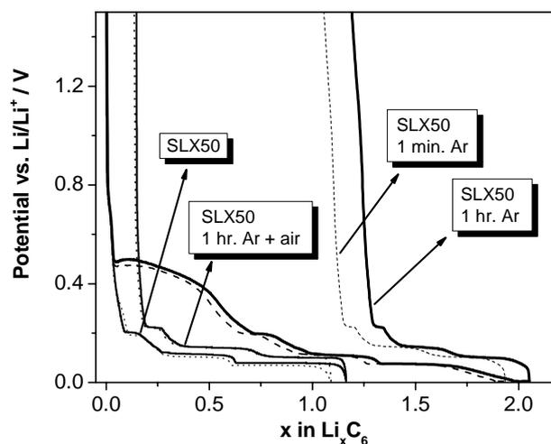
**Fig. 2:** First electrochemical lithium insertion into TIMREX<sup>®</sup> SLX50 (i) as received and (ii) heat treated at 1300°C in argon for 1 min and 1 h, respectively, and subsequently cooled down in argon and air atmosphere, respectively, in EC:DMC, 1M LiPF<sub>6</sub> electrolyte.
