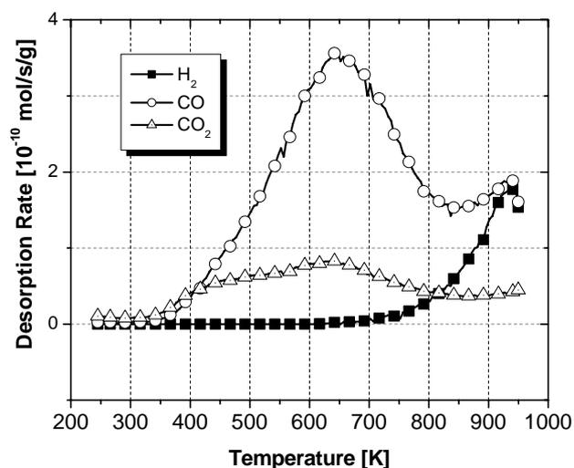
**Fig. 1:** Desorption rate of CO and CO<sub>2</sub> as a function of desorption temperature after oxygen chemisorption, for the “SLX50 1hr Ar” sample.
