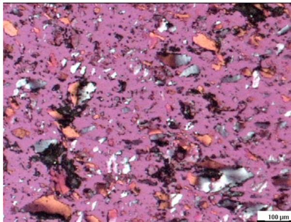
**Figure 3.** Optical micrograph of the RBSC material produced from PY-480-5-160. Image taken using polarized light.
