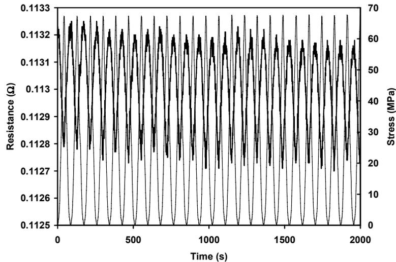
Figure 2. Variation of the longitudinal volume resistance (at the stressed region) (thick curve) with time and of the through-thickness compressive stress (thin curve) with time during through-thickness stress cycling of a quasi-isotropic carbon fiber epoxy-matrix composite at a fixed stress amplitude of 67 MPa. (Wang, D. and Chung, in press))
