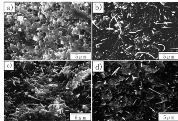
**Figure 4** The SEM micrographs of fracture surface of a)HP-A11300, b)HP-CNF1300, c)HP-CNF1400, d)HP-CNF1450.
