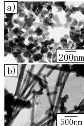
Figure 2 The TEM micrographs of a)Al<sub>2</sub>O<sub>3</sub> powder and b)carbon nanofiber
