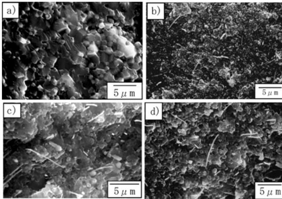
**Figure 3** The SEM micrographs of fractured surface of a)PL-A11300, b)PL-CNF1300, c)PL-CNF1400, d)PL-CNF1450.
