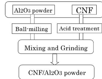
Figure1 Preparation process of CNF/Al<sub>2</sub>O<sub>3</sub> composite powder
