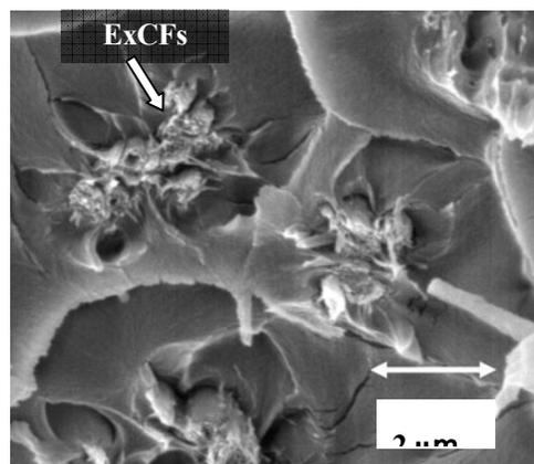
Figure 3. SEM micrograph of fracture surface of ExCFs/PMMA composite
