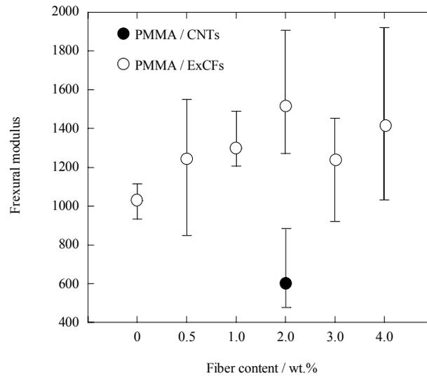
Figure 2. Dependence of fiber content of PMMA/ExCFs and PMMA/CNTs composite for flexural modulus
