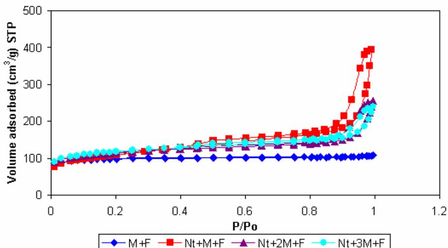
**Figure 2.** Nitrogen sorption/desorption isotherms at 77 K for NTs-composites.
