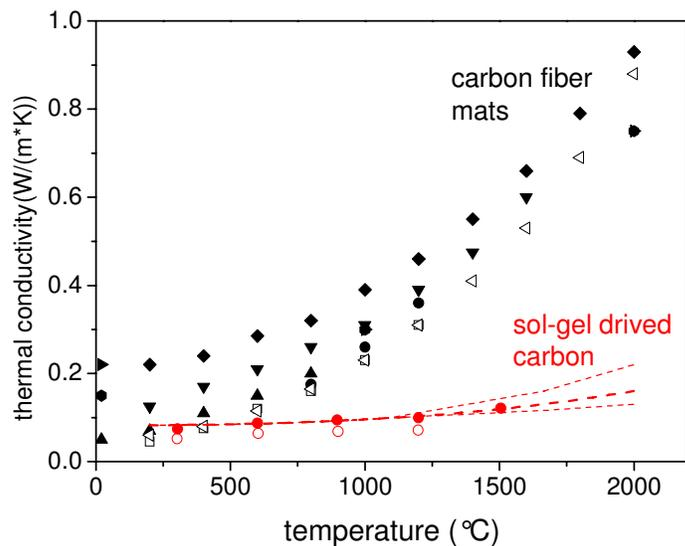
**Figure 2.** Total thermal conductivity of commercially available carbon fiber felts for thermal insulation (black symbols) and a carbon aerogel (red symbols). The closed symbols represent the thermal conductivity at ambient pressure, while the open symbols indicate the figures for the evacuated materials. The dashed lines in case of the aerogel mark the expected range in thermal conductivity at high temperatures where no experimental values are available yet.
