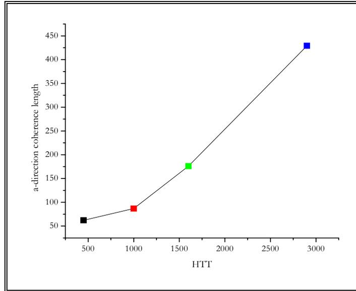
**Figure 3.** Graph showing increase in a-direction coherence length (calculated from the Raman spectrum from the binder of composites prepared from large flake graphite) with HTT
