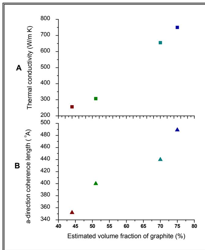
**Figure 4.** Plot of thermal conductivity of graphitized large flake composites (A) and a-direction coherence length of the binder (B) with varying estimated volume fraction of graphite
