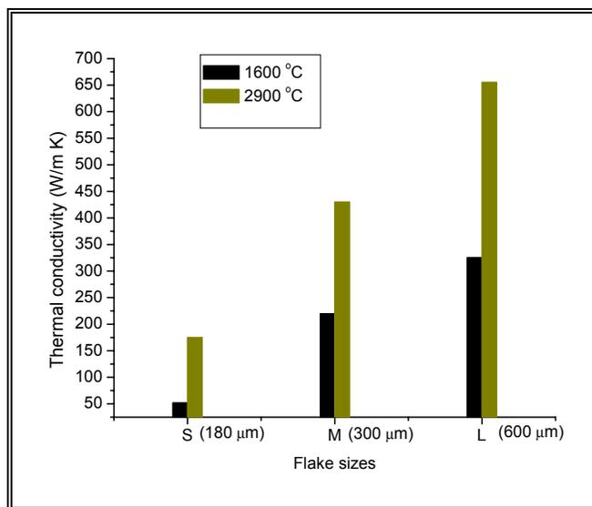
**Figure 1.** Thermal conductivity of composites of different flake sizes heat-treated to 1600 °C and 2900 °C
