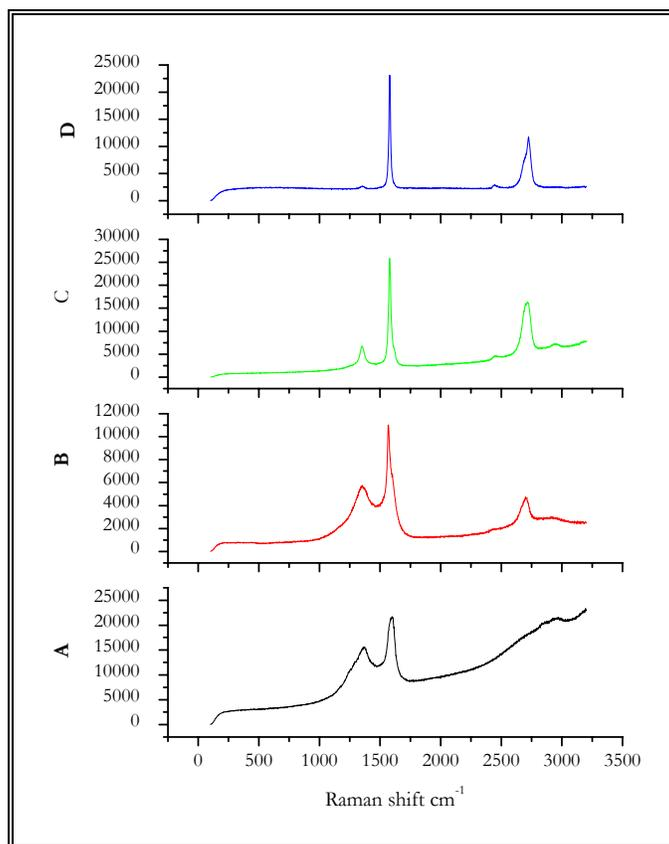
**Figure 2.** Raman spectra from the binder of samples prepared using large flake graphite at different HTT (A) as prepared, (B) carbonized to 1000 °C, (C) HTT 1600 °C and (D) graphitized (~2900 °C). The micrographs show the area of the sample at which spectra were acquired.
