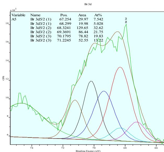
Figure 1. Br High-Resolution Scan of a Typical B-PAC<sup>TM</sup>
