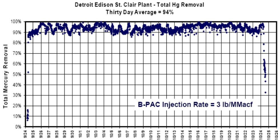
Figure 4. Total Mercury Removal of St. Clair 30-day Test
