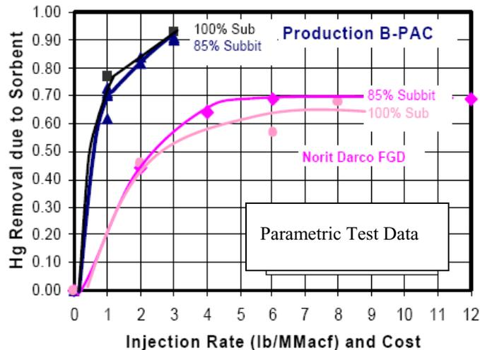
Figure 3. Mercury Removal due to Sorbent of St. Clair Test
