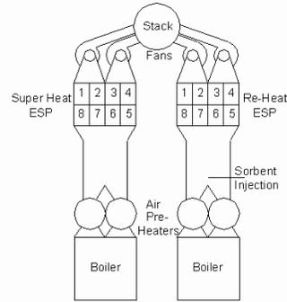
Figure 2. Overview and Duct Configuration of Midwest Generation’s Crawford Generation
