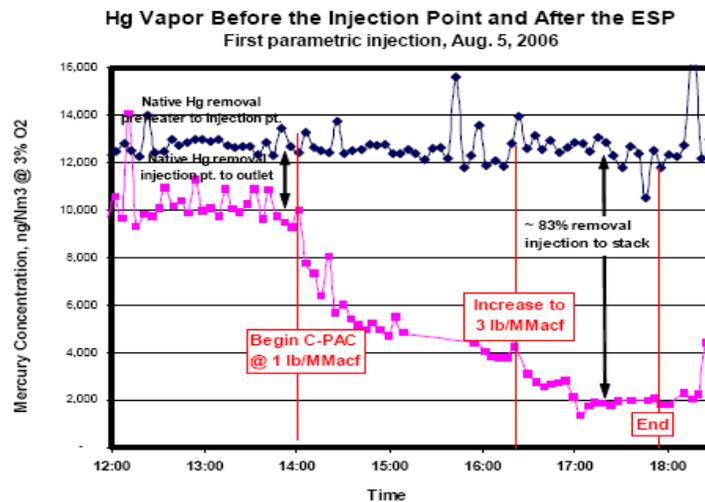
Figure 3. Hg Vapor Concentration before Injection Point and After ESP
