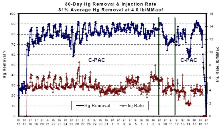
Figure 4. Hg Removal of 30-day Continuous Sorbent Inject Test in Crawford
