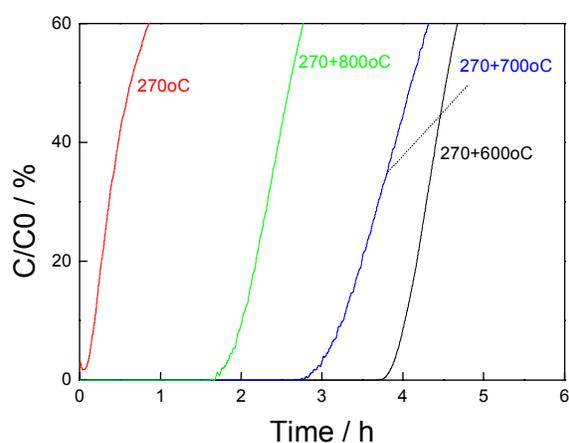
**Figure 3.** The formaldehyde adsorption behaviors of the stabilized PCNF and carbonized PCNFs
