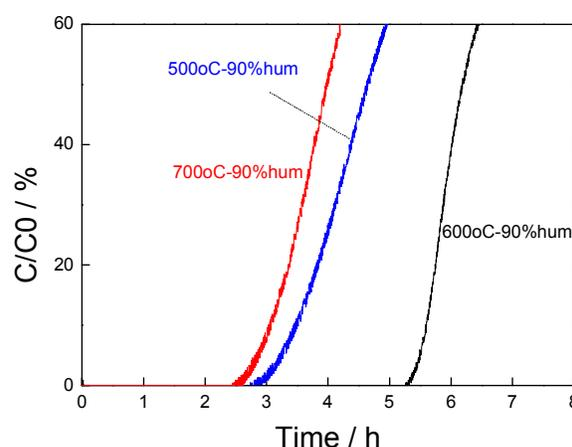
**Figure 4.** The formaldehyde adsorption behaviors of PACNFs.
