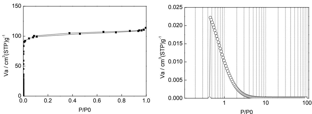
**Figure 1.** BET isotherms and pore sized distribution of PACNF.
