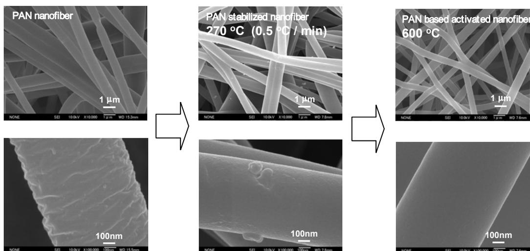
**Figure 2.** SEM images of PCNF, stabilized PCNF and PACNF.
