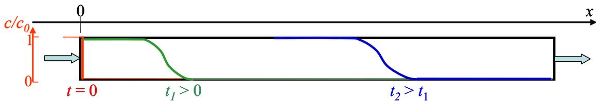
**Figure 1.** Propagation of the concentration front  $c/c_0 = f(x,t)$  through the adsorbent bed
