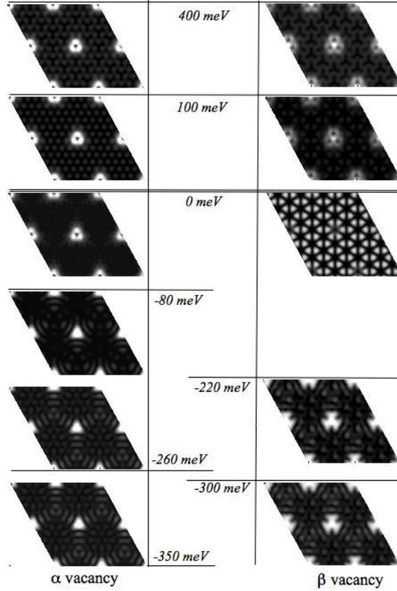
**Figure 4.** Calculated STM images for different domains in energy for the  $\alpha$  and  $\beta$  vacancies.
