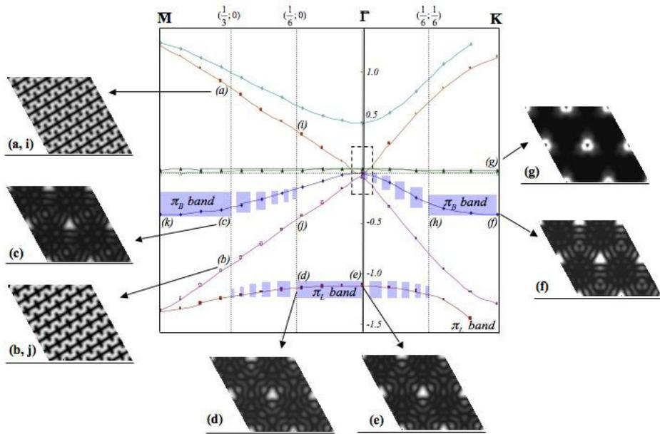
**Figure 2a.** The electronic band structure of the 6x6 model with an atomic vacancy on an A-type site in the center of the working cell. Cuts of the square modulus are shown as gray scale images are presented for some relevant point of the band structure from (a) to (k). The three-branch star feature of the  $\pi_B$  and  $\pi_L$  bands are shown as shaded areas.
