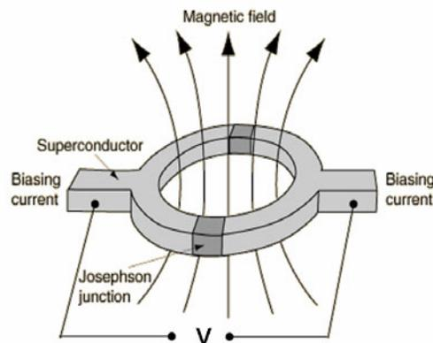
**Figure 1.** Principle of the SQUID sensing element.
