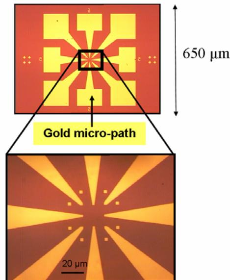
**Figure 2.** Sketch of the gold micro-path pattern deposited via optical lithography onto the doped Si wafers.
