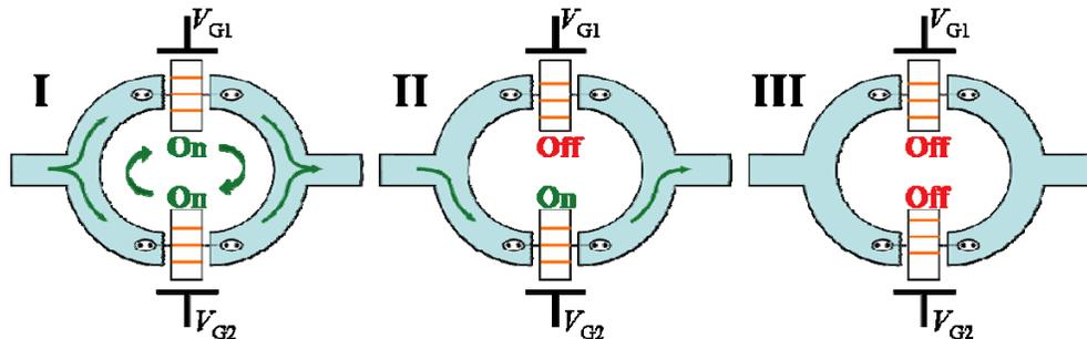
**Figure 4.** Sketches of the Nano-SQUID with two nanotube junctions, which can be tuned with the gate-voltages  $V_{G1}$  and  $V_{G2}$ . In case I, both junctions have a quantum level adjusted to the Fermi energy of the leads (on-resonance) and maximal supercurrent can flow through the device. In cases II and III, one and two junctions are tuned off-resonance, respectively.
