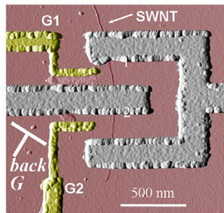
**Figure 3.** AFM image of a typical Nano-SQUID device. The three bimetallic contacts with the fork geometry make the SQUID loop (grey colour), in which the two uncoated portions of the SWNT (diameter  $\sim 1$  nm) between the contacts act as the two Josephson junctions (with length of about 200 nm) of the loop. In addition, Two lateral gates G1 and G2 (gold colour) are added in front of the Josephson junctions, in addition to the back gate which is the doped Si substrate itself.
