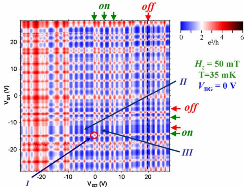
**Figure 5.** Correlation between normal-state conductance and superconducting switching current. Colour-scale representation of a typical differential conductivity  $dI/dV$  map at 35 mK and a backgate voltage  $V_{BG} = 0$  as a function of the lateral gate voltages  $V_{G1}$  and  $V_{G2}$ . A magnetic field of  $H_z = 50$  mT was applied perpendicular to the SQUID plane in order to suppress the superconductivity of the leads. The effect of cross-capacitance was subtracted in situ.
