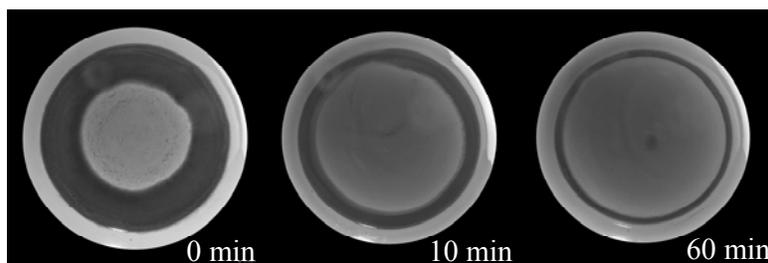
**Figure 5.** Photography of the sediments at the bottom of the flasks for 0, 10 and 60 minutes of ultrasonic stirring.
