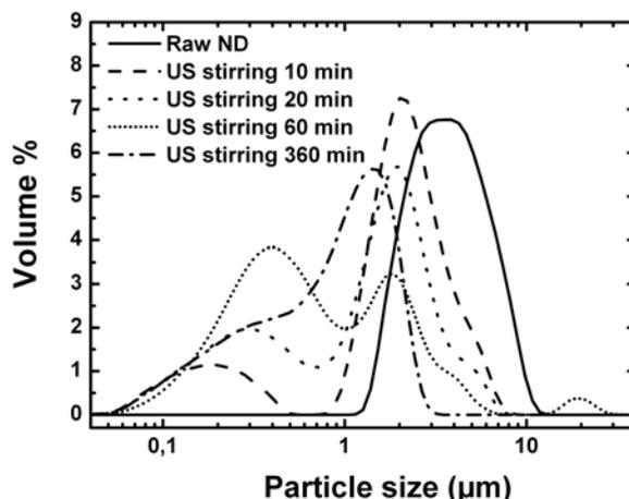
**Figure 4.** Particle size distribution of the suspensions treated by strong ultrasonic stirring.
