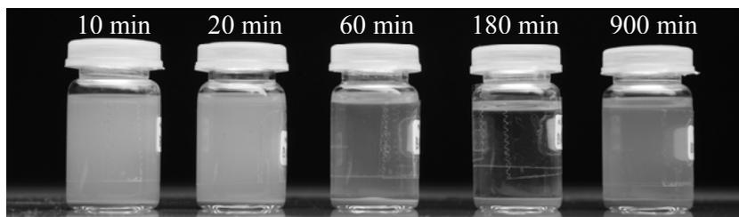
**Figure 1.** Photography of nanodiamonds suspensions obtained for different times of ball milling treatment after one day decantation.
