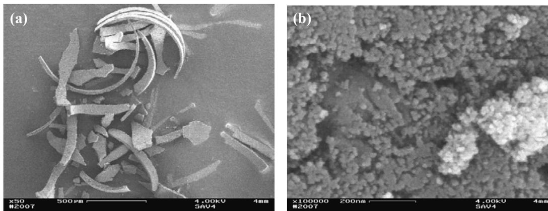
**Figure 2.** SEM images of the dried powder obtained after 60 minutes of ball milling treatment.
