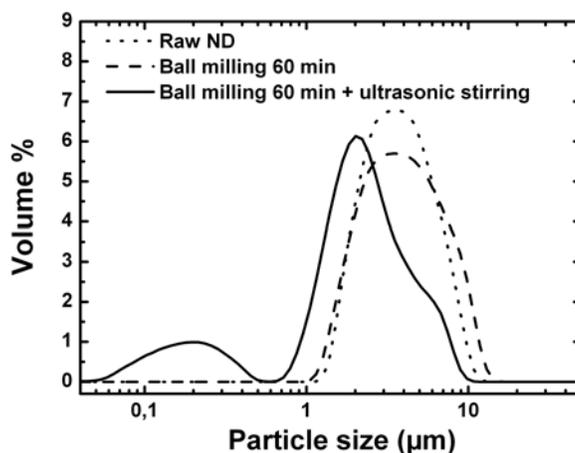
**Figure 3.** Particle size distribution of miscellaneous suspensions: raw nanodiamonds and suspensions treated during 60 minutes by ball milling without and with ultrasonic treatment.
