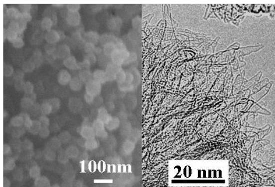
**Figure 1.** FE-SEM (Left) and TEM (Right) Images of as-grown Single-Wall Carbon Nanohorns.
