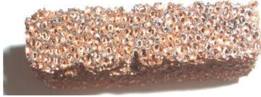
**Figure 2.** Cross sectional view of electrolessly plated graphite foam
