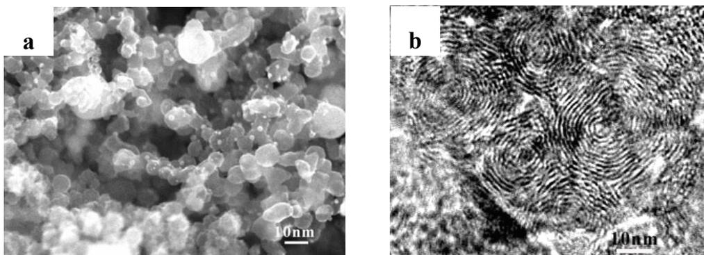
Fig.1 Images of carbon onions synthesized by arc-discharge in water. a)SEM, b)HRTEM.
