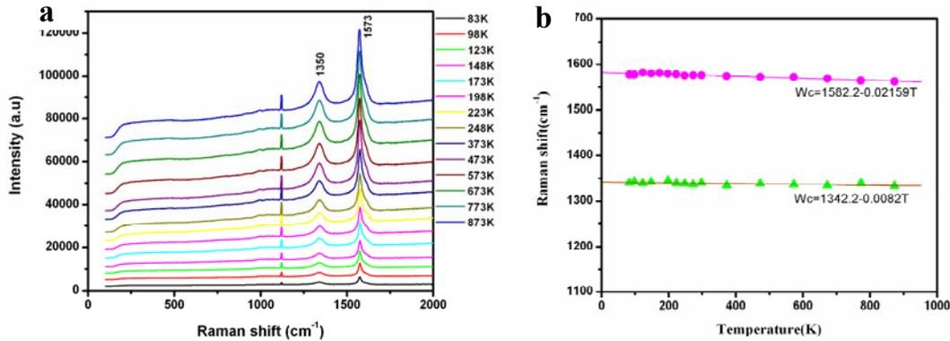
Fig.2 a) Raman spectra and b) the peak frequencies of D and G bands on temperature for carbon onions synthesized by arc-discharge in water.
