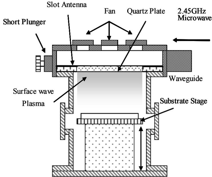
**Fig. 1** Schematic diagram of MW SWP CVD system.
