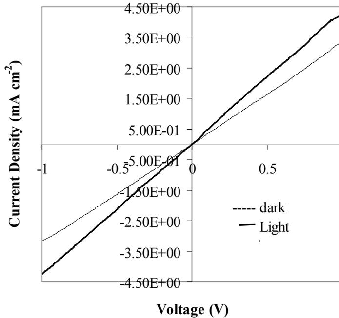
**Fig. 6** I-V characteristics of Au-a-C/ITO structure of the a-C thin film deposited at  $300\text{ }^\circ\text{C}$
