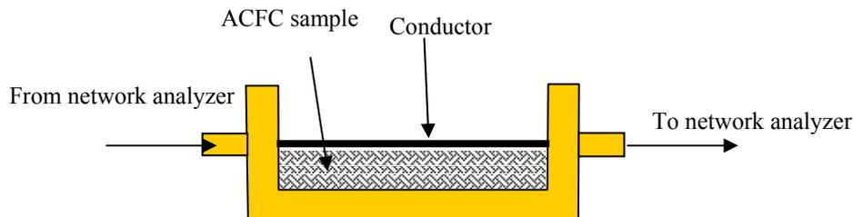
**Figure 1.** Setup for holding the ACFC sample for measurement of the microwave attenuation coefficient
