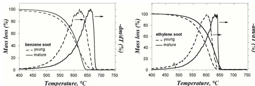
**Figure 5.** TG and DTG curves ( $10^{\circ}\text{Cmin}^{-1}$ ) under air ( $30\text{ ml min}^{-1}$ ) corresponding to benzene and ethylene soot.
