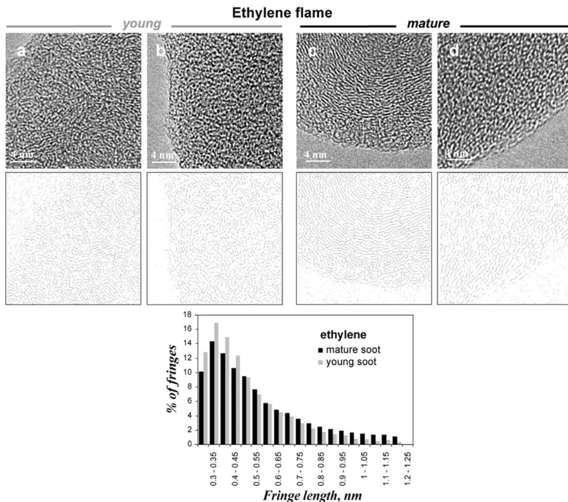
**Figure 4.** Raw HRTEM images (on the top) and corresponding skeletons below of young ethylene soot (left), mature ethylene soot (right) and relative histograms of fringe length.
