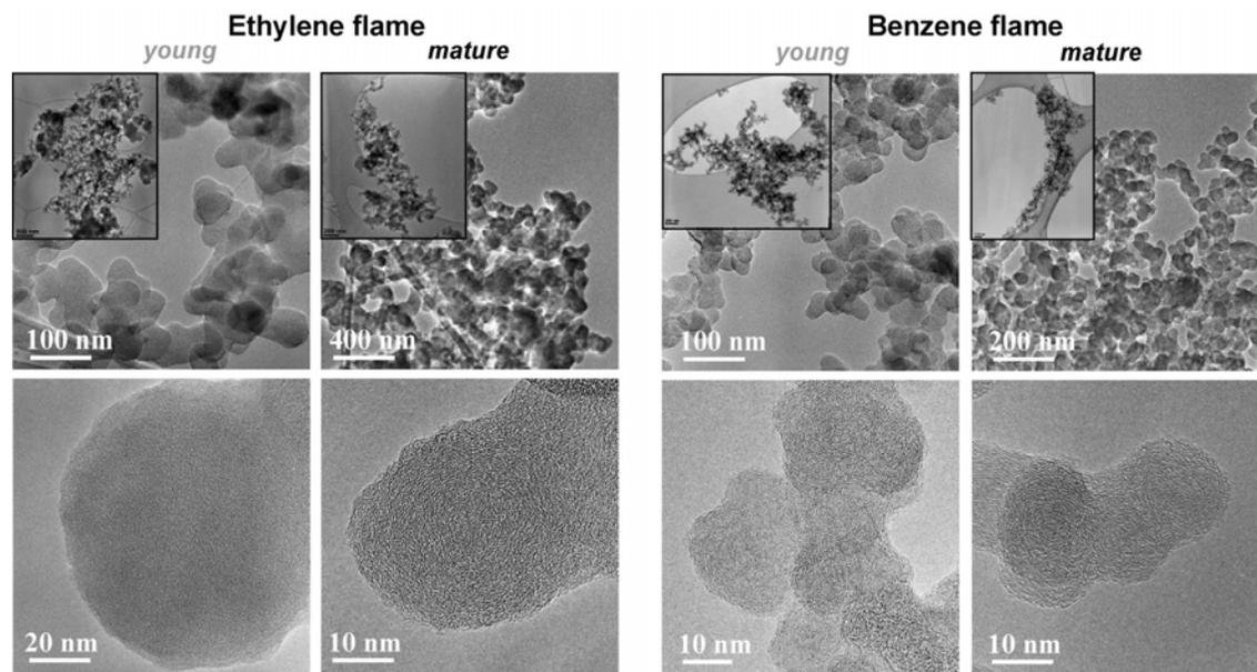
**Figure 1.** TEM and HRTEM of benzene (left) and ethylene soot (right).
