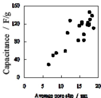
Figure 2. Dependence of EDLC capacitance on average pore size of ExCFs
