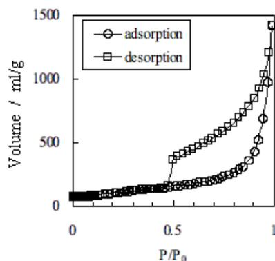
Figure 1. N<sub>2</sub> adsorption/desorption isotherm of exfoliated carbon fiber prepared from carbon fiber heat-treated at 2800 °C
