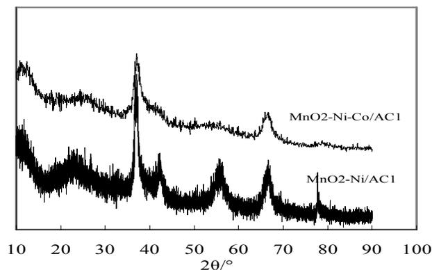
**Figure 2.** The XRD diffraction patterns of MnO<sub>2</sub>-Ni/AC1 and MnO<sub>2</sub>-Ni-Co/AC1
