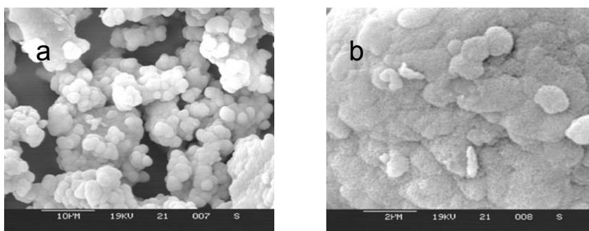
**Figure 3.** SEM images of MnO<sub>2</sub>-Ni/AC1)
