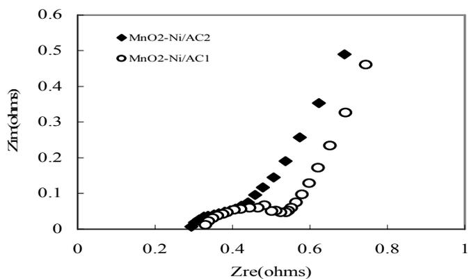
**Figure 5.** Nyquist plots of MnO<sub>2</sub>-Ni/AC1 and MnO<sub>2</sub>-Ni/AC2
