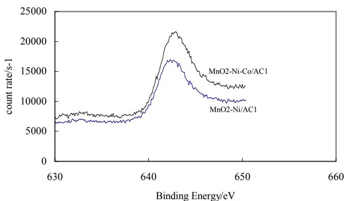
**Figure 1.** The XPS spectra for Mn2p<sub>3/2</sub> orbit of MnO<sub>2</sub>-Ni/AC1 and MnO<sub>2</sub>-Ni-Co/AC1
