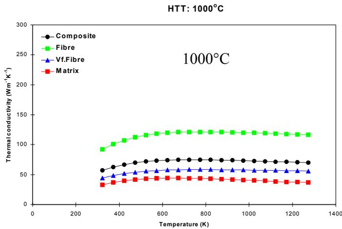
Figure 5. Thermal conductivity in the fibre direction of 1D C/C composites as a function of measurement temperature, compared with the measured values of the fibre and calculated values of the matrix for two HM PAN-based fibre/mesophase pitch matrix composites heat treated to 1000°C (top) and 2400°C (bottom).
