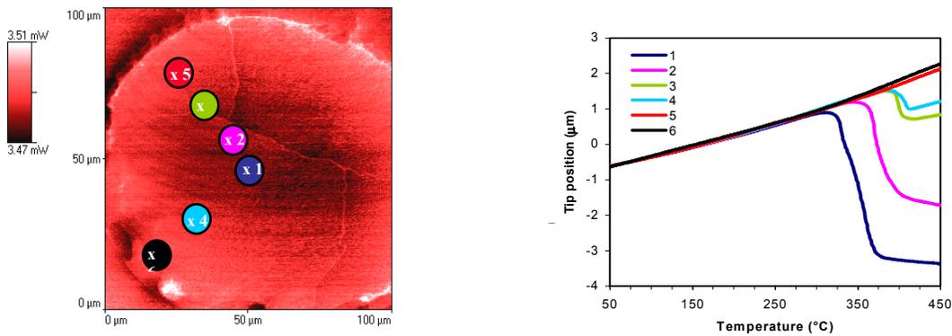
Figure1. Micro-thermal analysis data for a 100µm diameter mesophase-pitch fibre oxidised for 15h at 180°C in oxygen. The left hand micrograph is a thermal image; the dark regions are of lower thermal conductivity because they are of lower stabilisation degree. The right hand figure shows the softening behaviour at the various points indicated on the thermal image.
