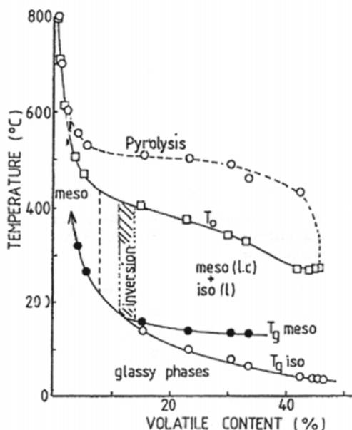
Figure 3. Pitch Transformation Diagram, showing the variation of glass transition temperatures with residual volatile content through the pyrolysis from isotropic pitch to mesophase to carbon. The two separate  $T_g$ s in the two phase region are shown.
