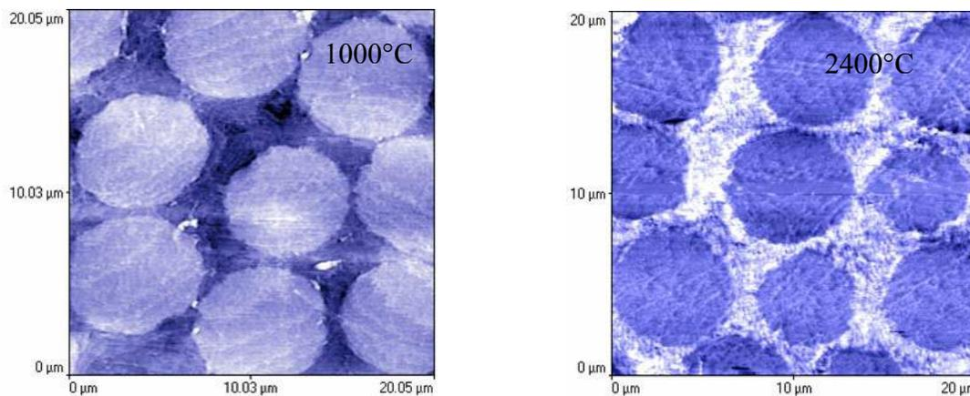
Figure 6. Thermal images of the 1000 and 2400°C C/C composites. The degree of brightness reflects the relative thermal conductivity.
