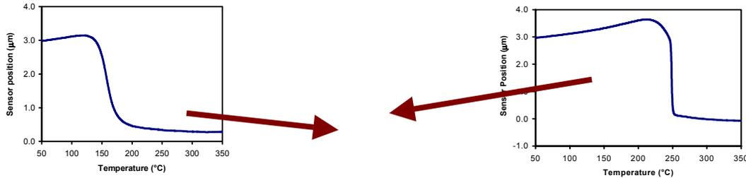
Figure 4. Microthermal analysis of two phase pitch showing the different softening behaviour of the mesophase sphere and the isotropic phase.
