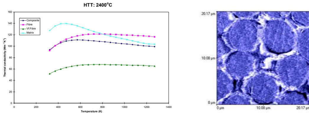
Figure 7. a) Thermal conductivity data in the fibre direction for a 1D C/C composite, the corresponding fibres and calculated values for the matrix. The fibres are High modulus PAN-based and the matrix is derived from a phenolic resin.
