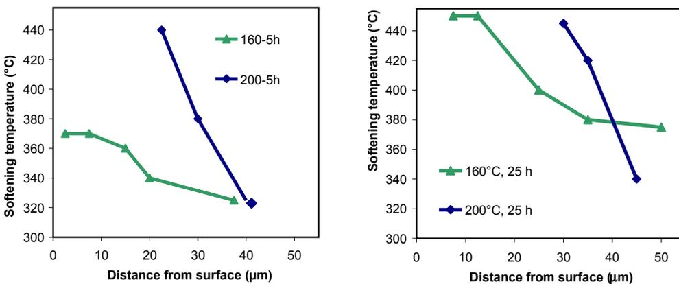
Figure 2. Softening temperature profiles for 100µm diameter mesophase-pitch fibres oxidised for 5 and 25h in oxygen at 160 and 200°C.
