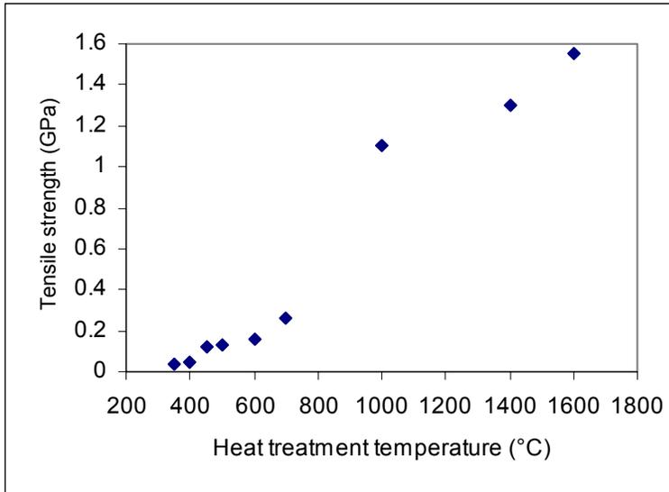
Figure 4. Tensile strength vs. heat treatment temperature of carbon tapes
