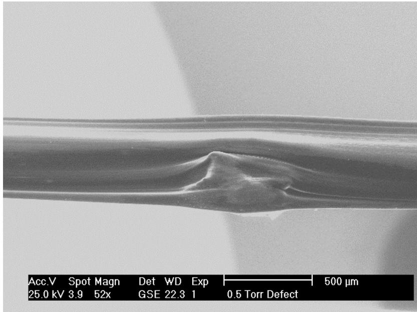
**Figure 11. Nodes on the tape surface**
