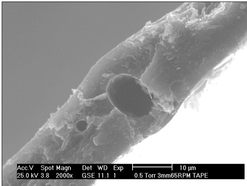
**Figure 13. Pore within carbon tape resulting from air / gas entrapped during “melting” of the pitch precursor**
