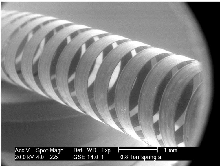
Figure 5. Scanning electron micrograph of continuous carbon tape spring
