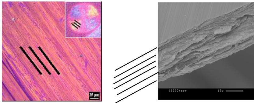
Figures 2 and 3. Optical and scanning electron micrographs of transverse sections of carbonised tapes
