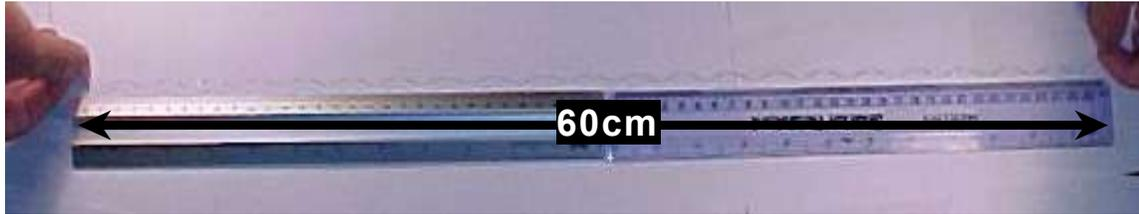
**Figure 6. Demonstration of the elastic extensibility of the tape springs**
