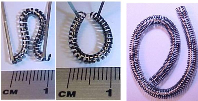
**Figure 7. Demonstration of flexibility exhibited by carbon tape springs**
