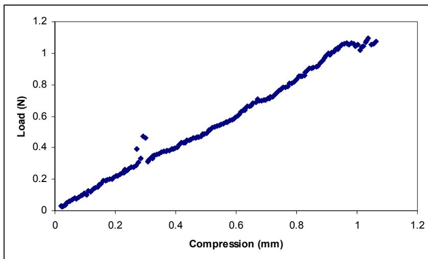
**Figure 10. Radial compression vs. load for 0.70 mm wide spring**
