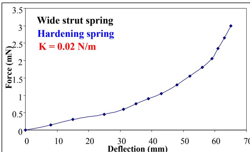
**Figure 8. Longitudinal extension vs deflection of 0.70mm wide carbon tape spring**
