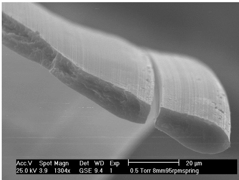
**Figure 12. Striation lines on the face of tape cause the tape or spring split along its length**
