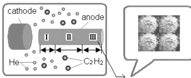
**Fig. 1** Schematic illustration of arc-assisted CVD experiments for making novel micro-sized carbons.
