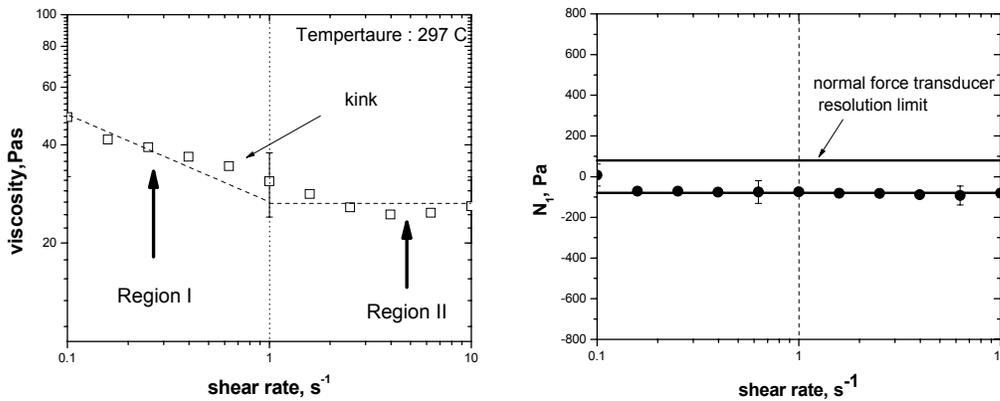
Figure 1: Viscosity and primary normal stress difference ( $N_1$ ) vs. shear rate for AR-HP mesophase pitch at a temperature of 297°C
