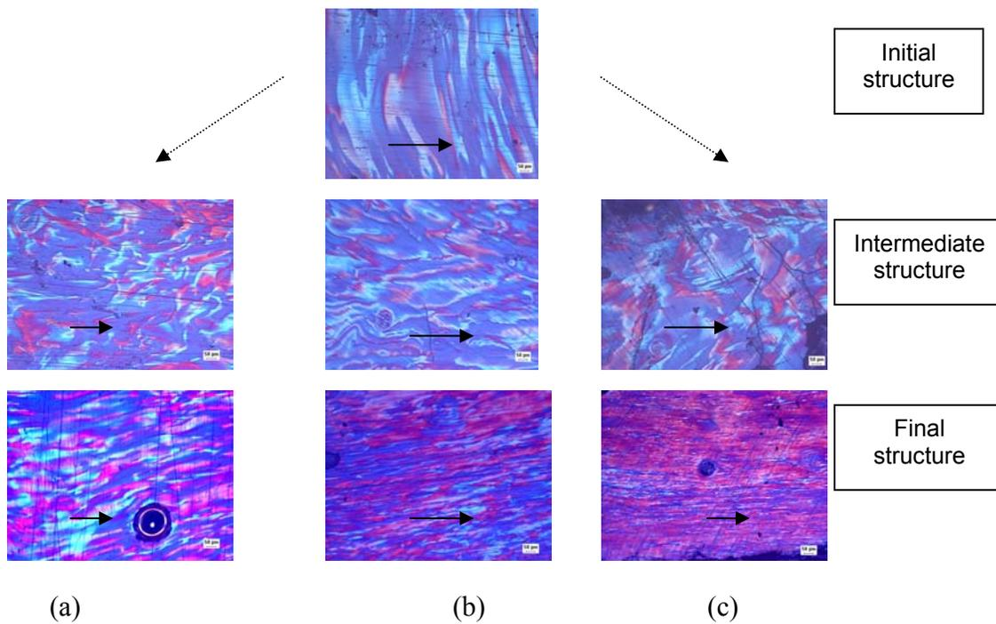
Figure 5: Evolution of microstructure for AR-HP mesophase pitch at 297C at shear rates of (a)  $0.1 \text{ s}^{-1}$ , (b)  $1 \text{ s}^{-1}$ , (c)  $10 \text{ s}^{-1}$  (the arrow  $\rightarrow$  represents flow direction)
