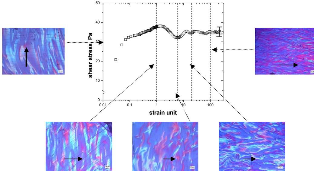
Figure 4: Rheological and microstructural data for AR-HP pitch at a shear rate of  $1 \text{ s}^{-1}$  (the arrow  $\uparrow$  represents the radial direction of the cone-plate fixture and the arrow  $\rightarrow$  represents flow direction)
