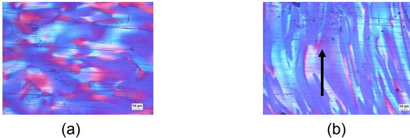
Figure 3: Microstructure of a) annealed sample; (b) after 5 minutes of waiting with cone and plate together (the arrow  $\uparrow$  shows the radial direction of the plate)
