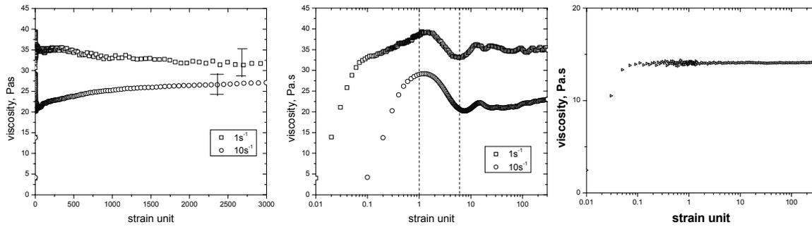
Figure 2: Transient rheological responses for the shear rates of  $1\text{s}^{-1}$  and  $10\text{s}^{-1}$  plotted in: a) linear scale, b) semi-log scale for AR-HP and c) for calibration fluid
