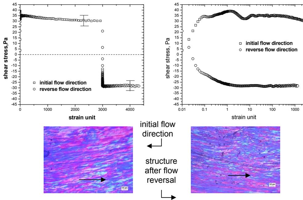
Figure 6: Typical shear stress response of AR-HP to flow reversal experiment at a shear rate of  $1 \text{ s}^{-1}$ . Also illustrated is the microstructure after flow reversal experiment, compared to a steady state microstructure (the arrow  $\rightarrow$  represents flow direction)
