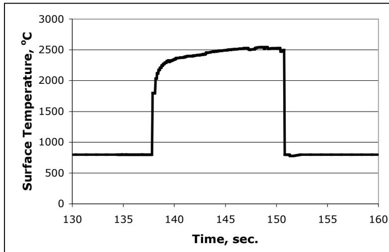
Figure 3. Example of surface temperature rise during the arc jet test of a CCA-3/SC1008 TWCP composite tested at  $750 \text{ W/cm}^2$  for 13 sec.
