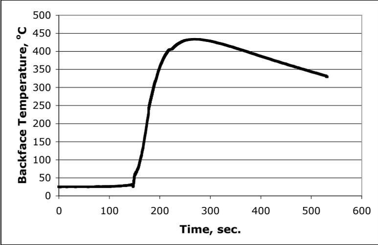
Figure 1. Example of backface temperature response during the arc jet test of a Lyocell/SC1008 TWCP composite at 1500 W/cm<sup>2</sup> for 7 sec.
