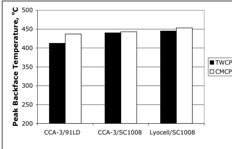
Figure 2. Summary of peak backface temperatures for different carbon phenolic composites tested at  $1500 \text{ W/cm}^2$  for 7 sec.
