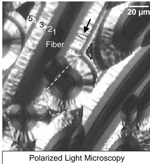
Figure 1. PLM micrograph of a polished section of an infiltrated carbon fiber felt. The matrix material consists of "cells" (one cell is marked by the dashed polygon) consisting of five ring-shaped layers (1-5) around one carbon fiber.
