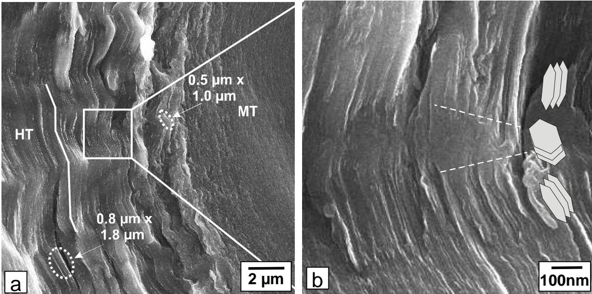
Figure 4. SEM micrographs of the fracture surface of the composite showing (a) zig-zag shaped lamellae within the HT layer and (b) regions with varying roughness within a lamellae. The two dashed ellipses in (a) show sections without bends within a lamellae.
