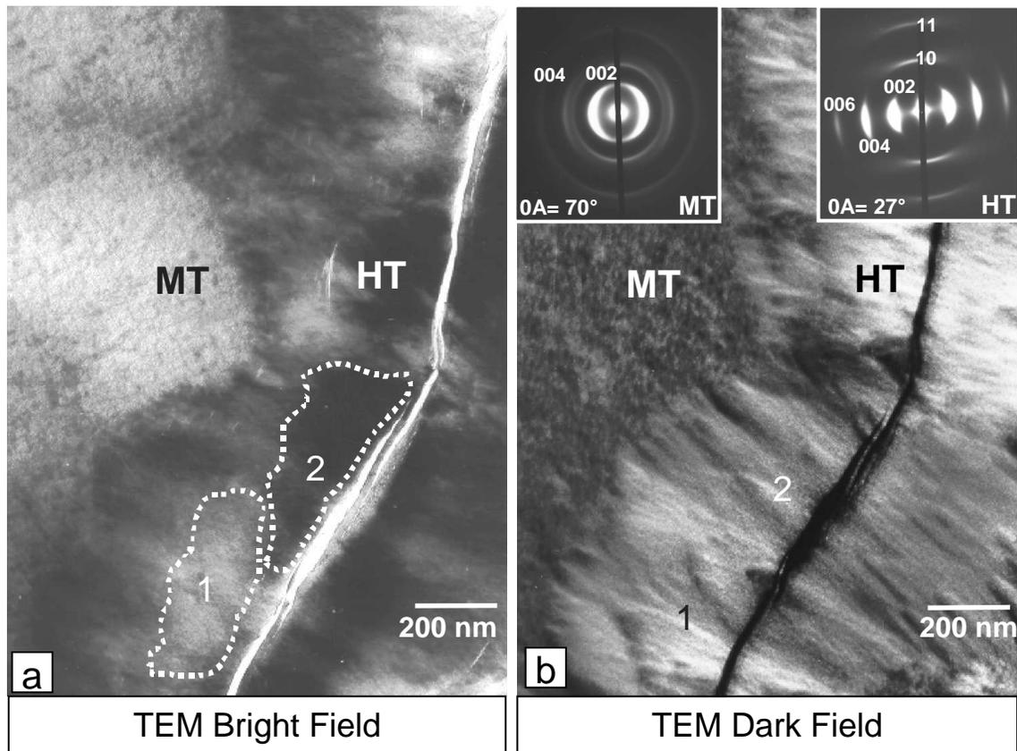
Figure 3. Microstructure of a TEM foil (after polishing, dimpling and ion etching) of the interfacial area between MT and HT layer: (a) TEM bright field image, (b) TEM (00.2) dark-field image (with SAED patterns derived from the MT and HT layers as insets) of the interfacial area between MT and HT layers. The white dotted lines in (a) mark two differently oriented domains.
