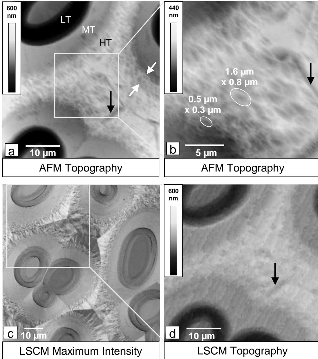
Figure 2. (a, b) AFM topography and (c, d) laser scanning confocal microscopy (LSCM) images of an infiltrated carbon felt after ion etching, (c) LSCM maximum intensity image, (d) LSCM topography image of the same region as shown in (a).
