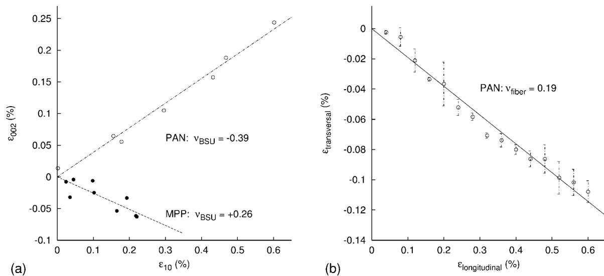
Figure 2 Poisson-ratio of (a) the nanocrystallites (BSUs), (b) of the whole carbon fiber
