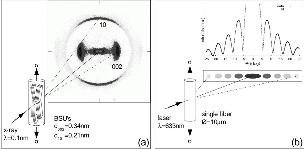
Figure 1 Sketch of the experimental setups and the obtained scattering images: (a) using synchrotron radiation, (b) using laser light
