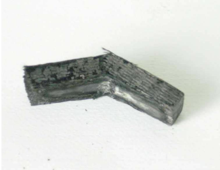
Figure 4. Images of fracture surface of 3D textile C/PyC/SiC composites
