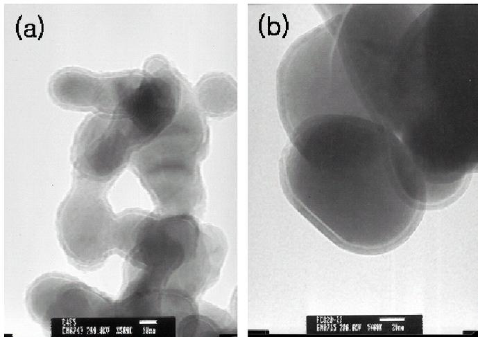
Fig.1. TEM images of Fe(C) nanocapsules with core-shell structure at different reaction temperatures; (a) 500°C, (b) 1100°C
