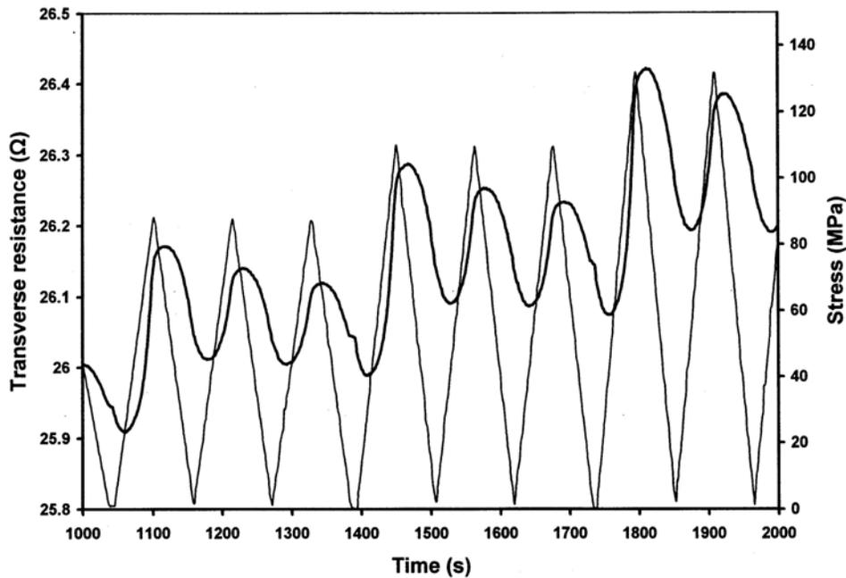
Fig. 6 Magnified view of a part of Fig. 5. extent of fiber-fiber contact in the through-thickness direction. After the reloading had reached an intermediate level, the resistance started to increase, due to fiber spreading. In other words, there were two microstructural effects, i.e., fiber spreading in the transverse direction and fiber squeezing in the through-thickness direction. Fiber spreading was the dominant phenomenon, but both phenomena occurred in each stress cycle.
