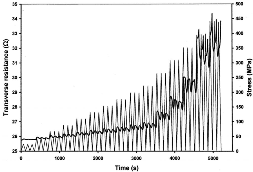
Fig. 5 Variation of the transverse volume electrical resistance with time (thick curve) and of the stress with time (thin curve) during stress cycling at progressively increasing stress amplitudes up to 450 MPa. Fracture was observed at the end of this test.
