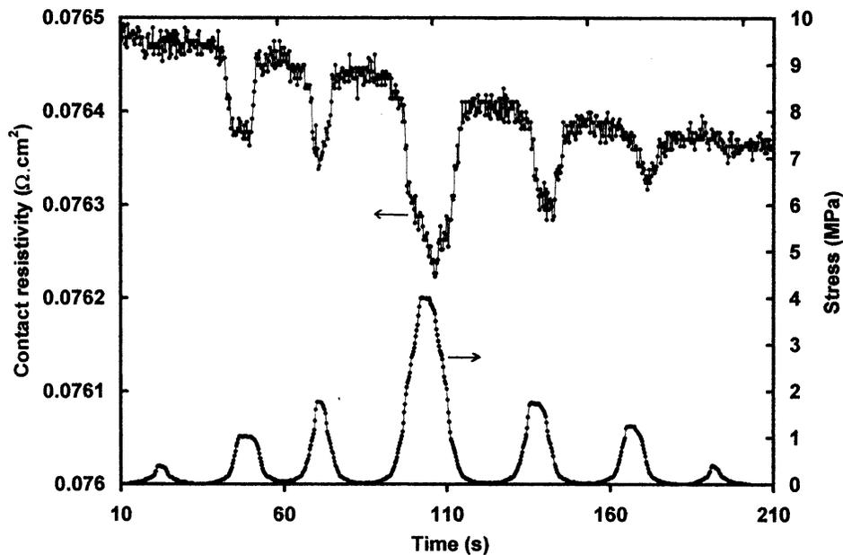
Fig. 3 Variation of the contact electrical resistivity with time and of the stress with time during stress cycling to different stress amplitudes up to 4 MPa. The specimen configuration is that in Fig. 1.
