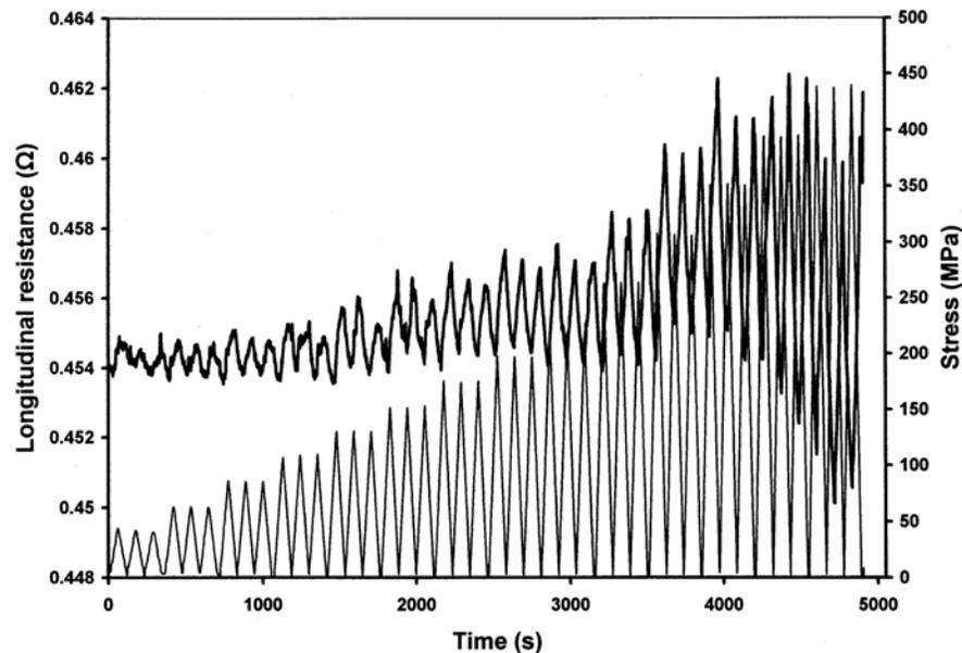
Fig. 4 Variation of the longitudinal volume electrical resistance with time (thick curve) and of the stress with time (thin curve) during stress cycling at progressively increasing stress amplitudes up to 450 MPa. Fracture was observed at the end of this test.
