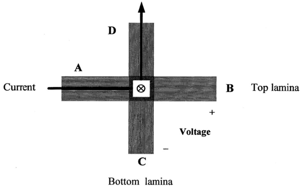
Fig. 1 Composite configuration for measuring the contact electrical resistivity of the interlaminar interface. A and D are current contacts; B and C are voltage contacts.
