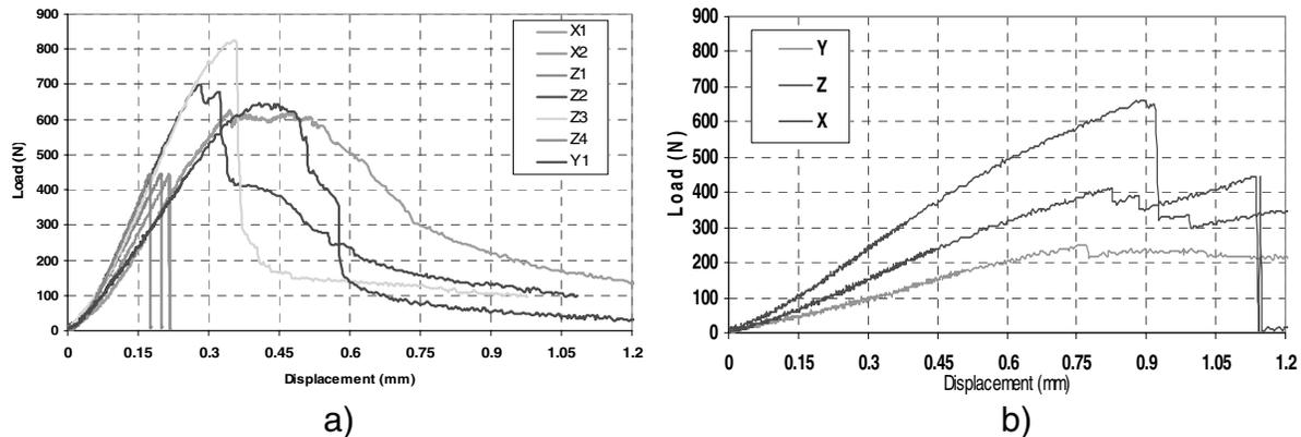
Figure 5. Load – displacement dependences as detected in four point bending tests for 2D (a) and 3D (b) material.
