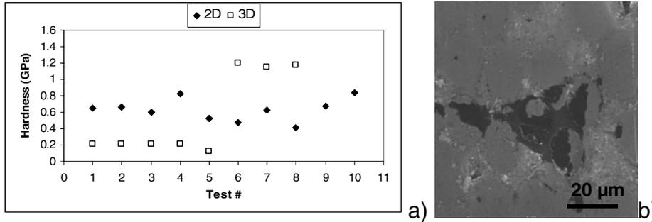
Figure 4. Nanoindentation results (a) and characteristic indent shape (b).
