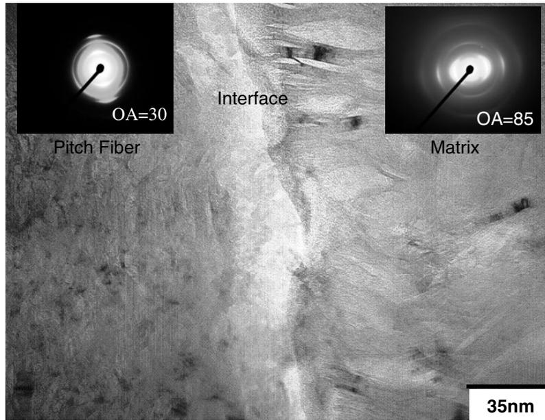
Figure 3a. TEM bright field image of 2D material. The inserts represent SAED patterns from the fiber (left part of the image) and matrix (right part) areas, respectively.
