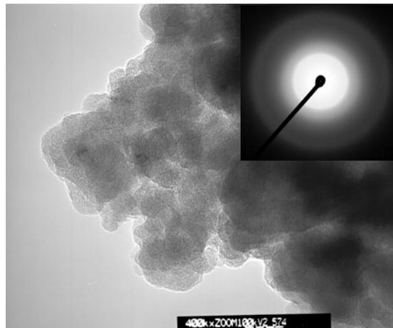
Figure 8. Bright field TEM image of an amorphous friction layer generated on the surface of 3D sample. Insert represents the diffraction pattern taken from the central part of the layer.
