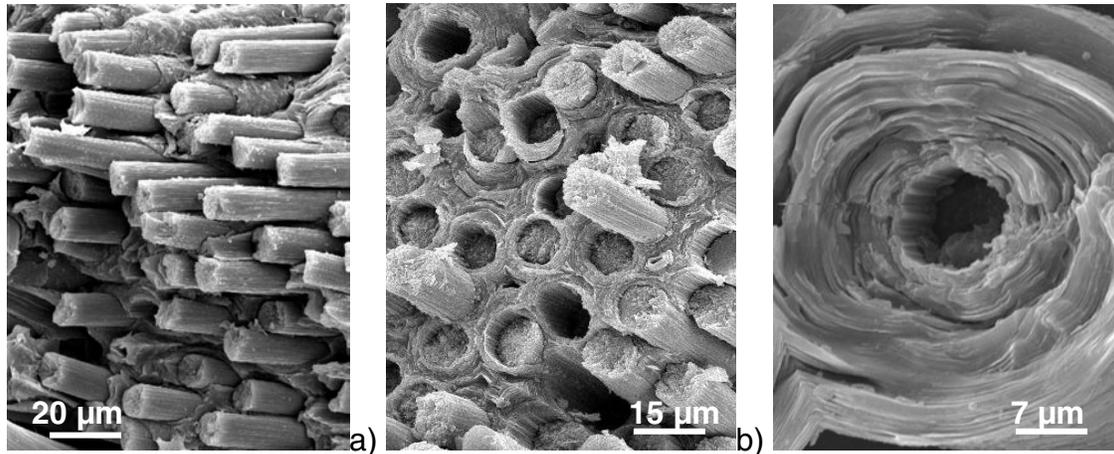
Figure 6. The fracture surface of 2D sample (a) and 3D sample (b) and detail in (c).
