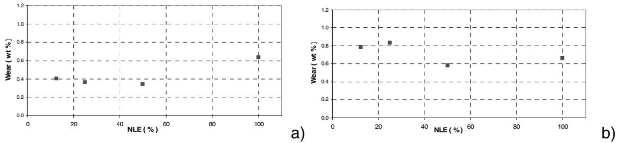
Figure 1. Wear of two investigated samples 2D (a) and 3D (b).
