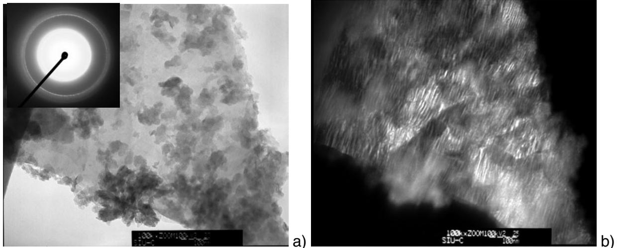
Figure 7. Bright field TEM image of semi-crystalline friction layer generated on the surface of 2D sample (a), diffraction pattern (insert in a) from the central part of (a), and dark field image (b).
