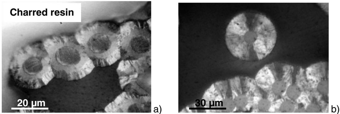
Figure 2. Microstructure of 2D (a) and 3D (b) material as seen in polarized light microscope.
