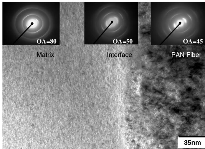
Figure 3b. TEM bright field image of 3D material. The inserts represent SAED patterns from the fiber (left part of the image) and matrix (right part) areas, respectively. A semi-crystalline interphase formed between C-fiber and CVI matrix.
