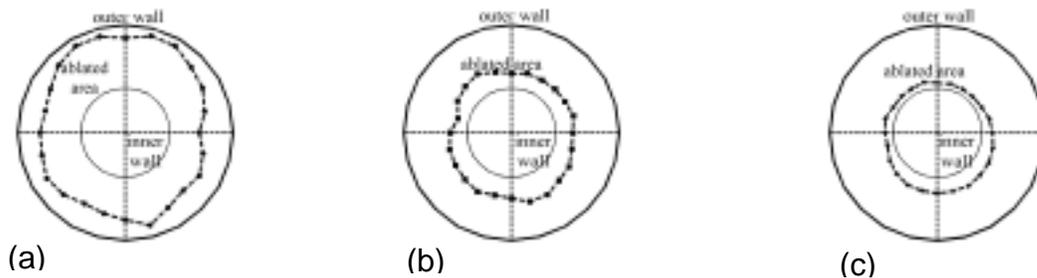
Fig. 1. Effect of pressure in the ablated area of the CFRC composites nozzle; (a) 0.1 MPa, (b) 60 MPa and (c) 90 MPa.
