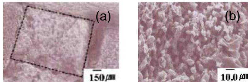
Fig. 7. SEM of the ablated carbon matrix in the CFRC composites prepared at 90 MPa.
