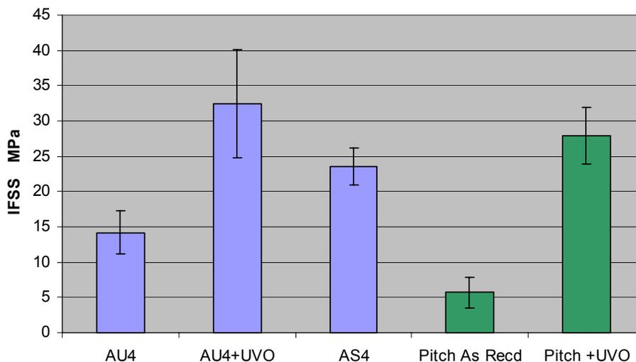
Figure 7. Interfacial shear strength from fragmentation test.
