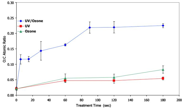
Figure 1. Effect of surface treatment on AU4 O:C atomic ratio
