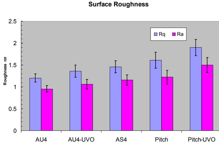
Figure 2. The effect of UVO treatment on carbon fiber surface roughness.
