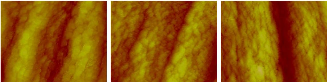
Figure 3. Typical STM images of AU4, AU4+UVO, and AS4 carbon fibers. X-Y scale collected at 300 nm, z range is 30 nm.
