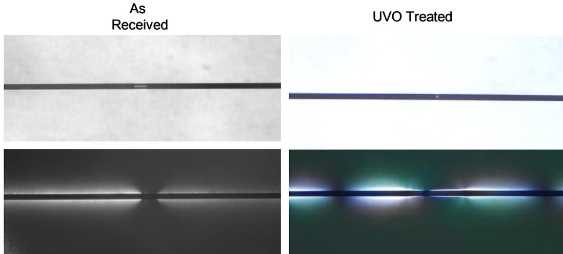
Figure 6. Failure mode of Dialead pitch fiber As Received (left) and UVO treated. Top photographs in transmitted light showing fiber fracture. Fiber diameter is nominal 12  $\mu\text{m}$ .
