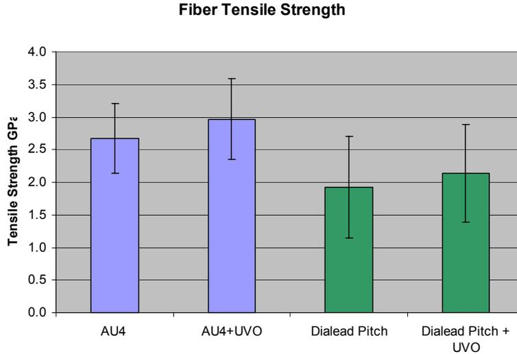
Figure 4. Single filament tensile strength.
