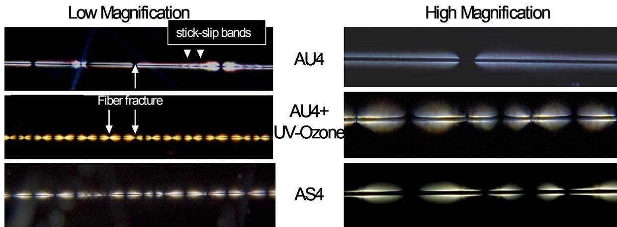
Figure 5. Birefringent stress pattern collected at high coupon strain showing differences in failure mode of AU4 (top), AU4+UV-Ozone (middle), and AS4. Fiber diameter is approximately 8  $\mu\text{m}$ .
