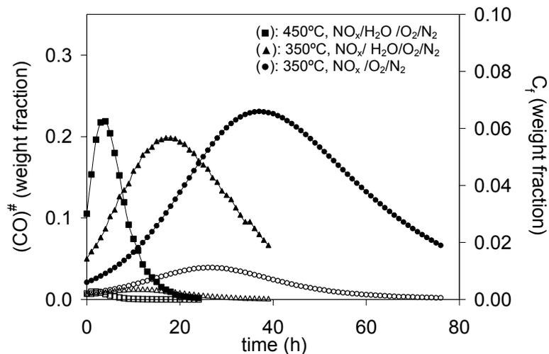
Figure 2. Predicted  $(\text{CO})^\#$  (solid symbols) and  $C_f$  (open symbols) profiles during selected lifetime tests with sample A3-16.8.
