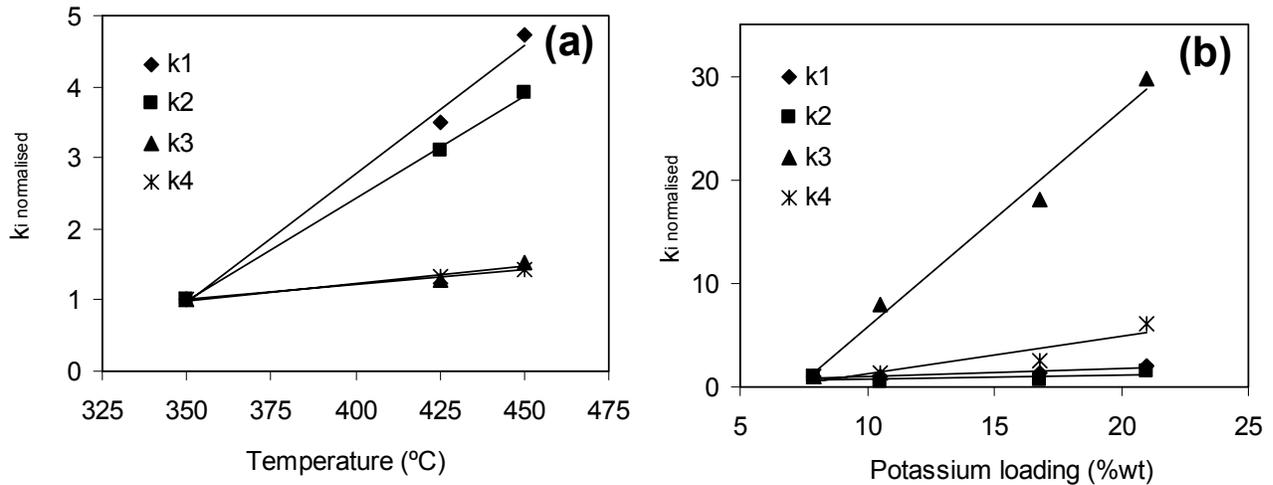
Figure 3 Normalised kinetic constants (reactive gas mixture  $\text{NO}_x/\text{O}_2/\text{N}_2$ ).
