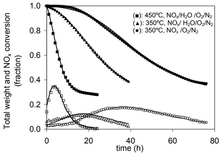
Figure 1. Total weight (solid symbols) and NO<sub>x</sub> conversion (open symbols) profiles during selected lifetime tests with sample A3-16.8. Symbols: experimental data; lines: model fittings.
