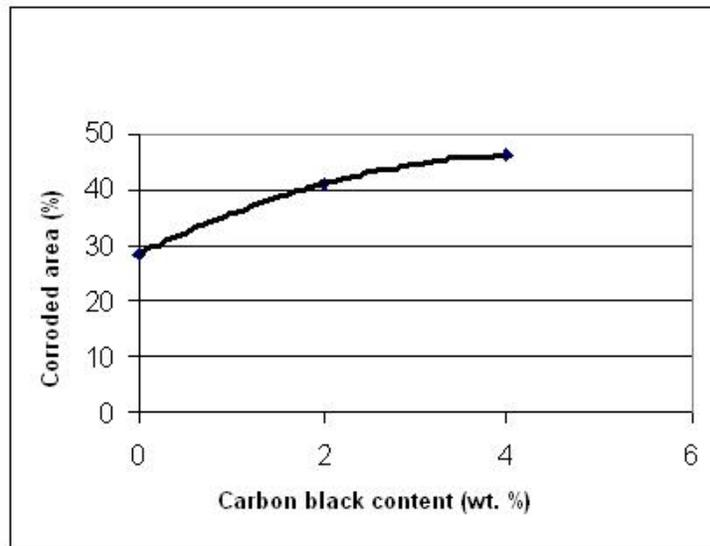
**Figure 7** Corroded area (%) of the metal surface against carbon black content in paint.
