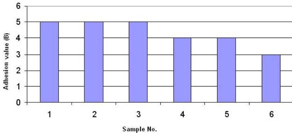
Fig. 1 Cross cut tests of graphite-containing paint.
