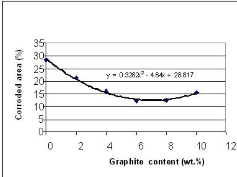
**Figure 6:** Corroded area (%) of the metal surface against graphite content in paint.
