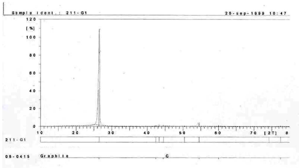
**Figure 8:** XRD pattern of the graphite
