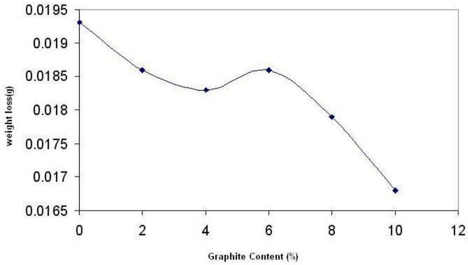
Fig. 3 Abrasion resistance of the graphite containing paints.
