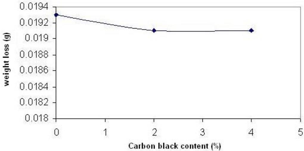
Fig. 4 Abrasion resistance of the carbon black containing paints.
