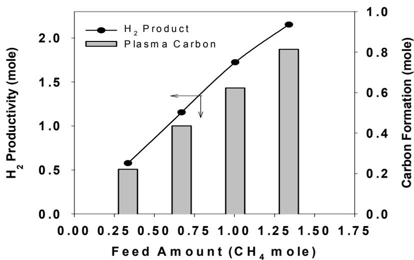
Figure 2. Effect of CH<sub>4</sub> feed on the yield of H<sub>2</sub> and carbon
