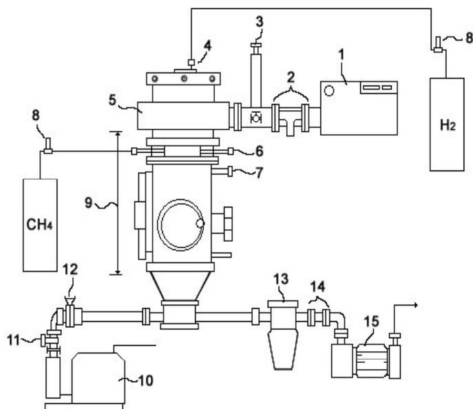
Figure 1. Experimental apparatus for microwave plasma and catalytic reaction system; (1) Magnetron, (2) Waveguide, (3) E–H tuner, (4) Microwave quartz tube, (5) Plasma Generator, (6) Jet inlet nozzle, (7) Cooling line inlet, (8) MFC, (9) Microwave plasma reactor, (10) Vacuum pump, (11,12) Control valve for pressure, (13) Cyclone, (14) Filter, (15) Mechanical diaphragm pump
