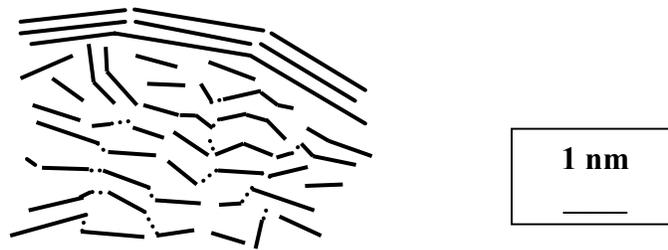
Figure 6. Sketch of the cross-section of a carbon fiber coated by pyrocarbon,
