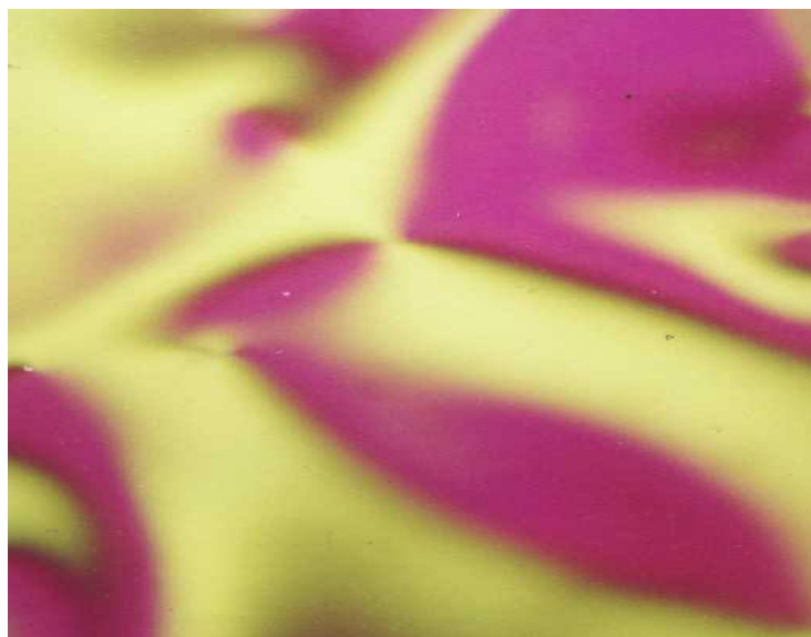
Fig. 4 Mesophase pitch polarize coarse fibrous structure
