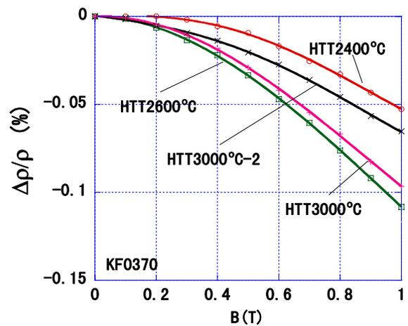
Fig. 3. Field dependence of maximum transverse magnetoresistance at 77K for phenol-based carbon fibers.
