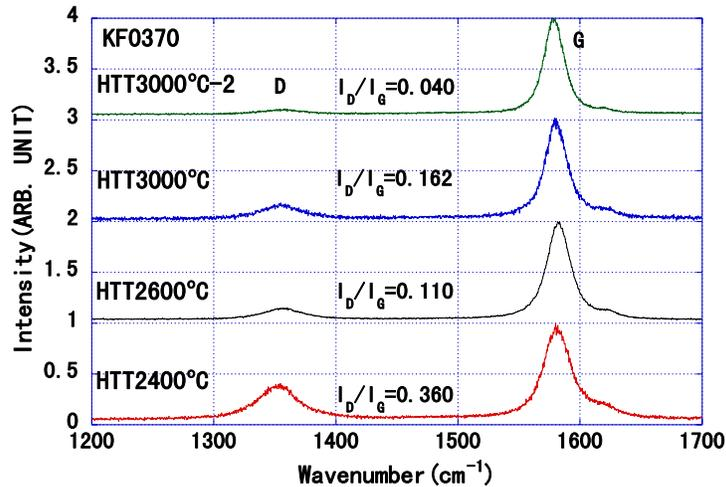
Figure. 4 First-order Raman spectra for phenol-based carbon fibers.
