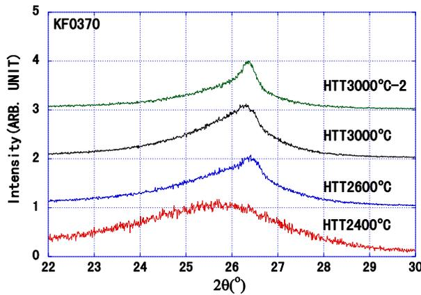
Fig. 2. X-ray diffraction patterns for phenol-based carbon fibers.
