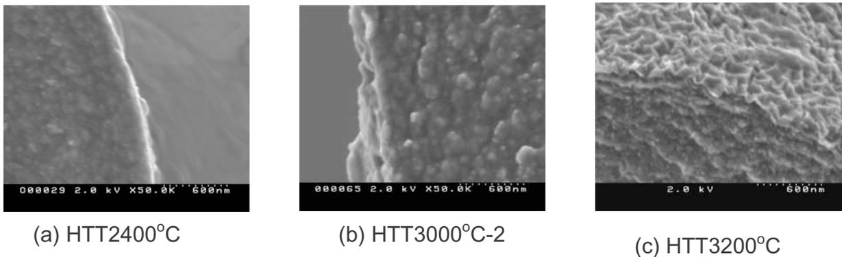
Fig.1 SEM images of cross sections of phenol-based carbon fiber fibers.
