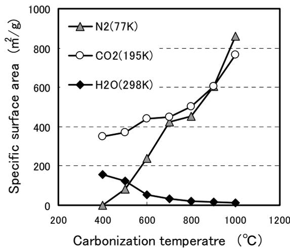
Figure 4. Temperature dependence of specific surface area of the charcoals estimated by N<sub>2</sub>, CO<sub>2</sub> and H<sub>2</sub>O.
