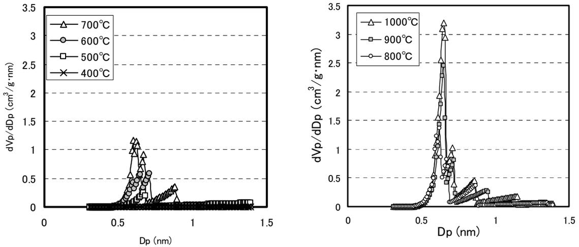
Figure 3. Distribution of pore radius of the charcoal estimated by N<sub>2</sub> adsorption at 77K
