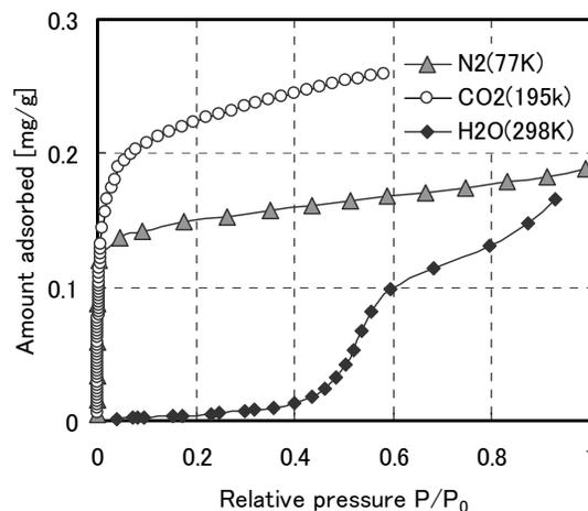
Figure 2. Adsorption Isotherms of  $N_2$ ,  $CO_2$  and  $H_2O$  for the charcoal carbonized at  $800^\circ C$
