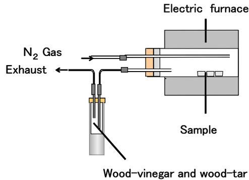
Figure 1. Apparatus for carbonization
