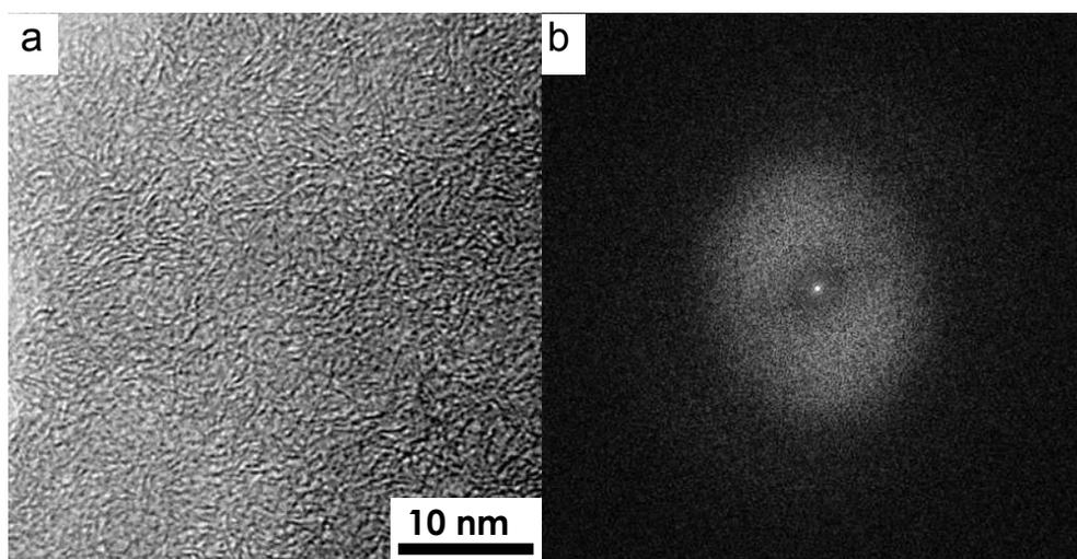
Figure 3. (a) HRTEM image of the carbon molecular sieve (sample KUA1B8), and (b) power spectrum of (a). Defocus value  $\Delta f$  is -60nm, Scherzer focus.
