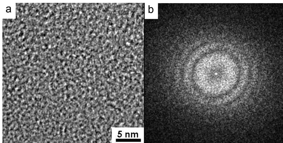
Figure 1. (a) HRTEM image of amorphous carbon film, and (b) power spectrum of (a) obtained by 2D-FFT. The defocus value  $\Delta f$  is -255nm.
