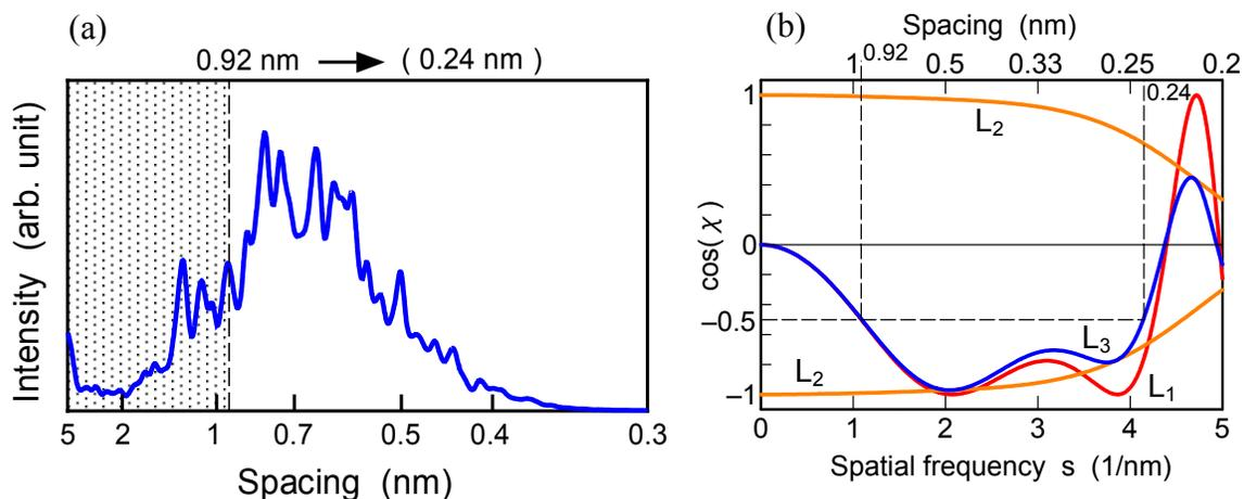
Figure 4. (a) Power spectrum of HRTEM image of the carbon molecular sieve (sample KUA1B8) obtained by 2D-FFT and (b). Phase transfer function of objective lens of the HRTEM. The defocus value  $\Delta f$  is  $-60\text{nm}$ . ( $L_1$ : the transfer function without attenuation obtained by equation (1),  $L_2$ : the damping envelope curves,  $L_3$ : the effective transfer function modified by the damping envelope function)
