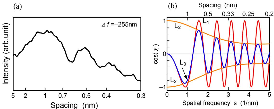
Figure 2. (a) Power spectrum of HRTEM image of amorphous carbon film obtained by 2D-FFT. (b) Phase transfer function of objective lens of the HRTEM. The defocus value  $\Delta f$  is  $-255\text{nm}$ . ( $L_1$ : the transfer function without attenuation obtained by equation (1),  $L_2$ : the damping envelope curves,  $L_3$ : the effective transfer function modified by the damping envelope function)
