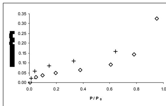
Figure 3. Adsorption and desorption of benzene at 303 K on T650.  $\diamond$ adsorption process, + desorption process
