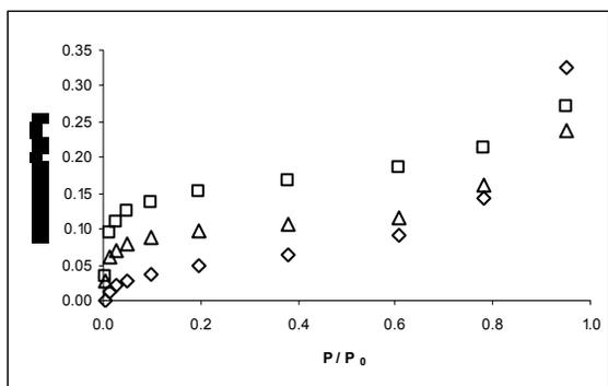
Figure 2. Adsorption of benzene at 303 K on:  $\diamond$ T650,  $\triangle$  T650-4,  $\square$  T650-8
