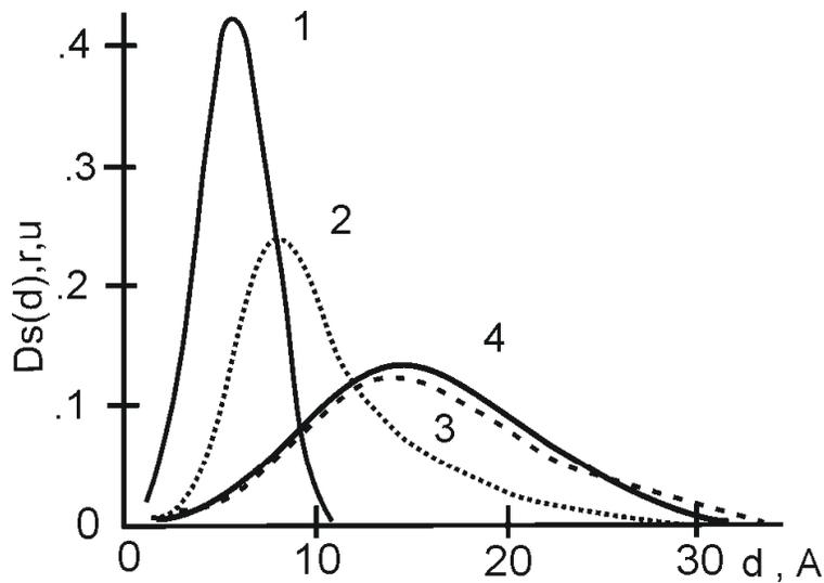
Figure 2. The distribution of inhomogeneities in the CF samples: 1 – CF with unimodal texture (activated by water steam at 500°C); 2 – CF with layered (bimodal) texture (treated by water steam at 600°C); 3,4 – oxidized pitch fibers (before carbonization and partial activation in water steam medium) oriented perpendicular and parallel to the X-ray beam, respectively.
