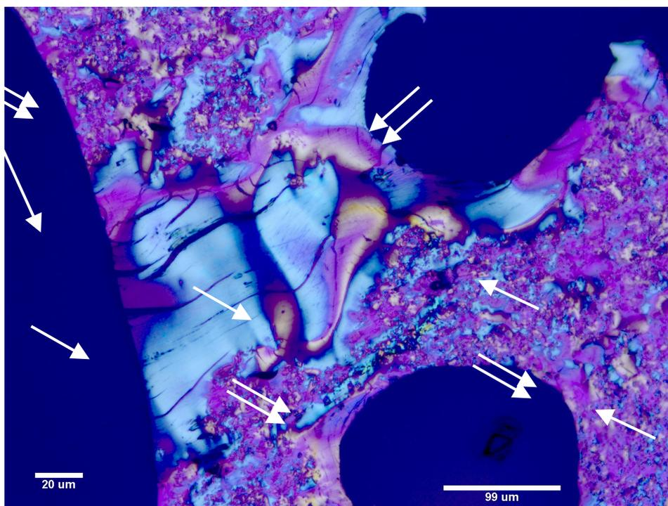
Figure 4. Large magnification optical micrograph of sample 40 showing variation anisotropy variations. Single arrows indicate areas free of nanotubes and double arrows are areas rich of nanotubes.
