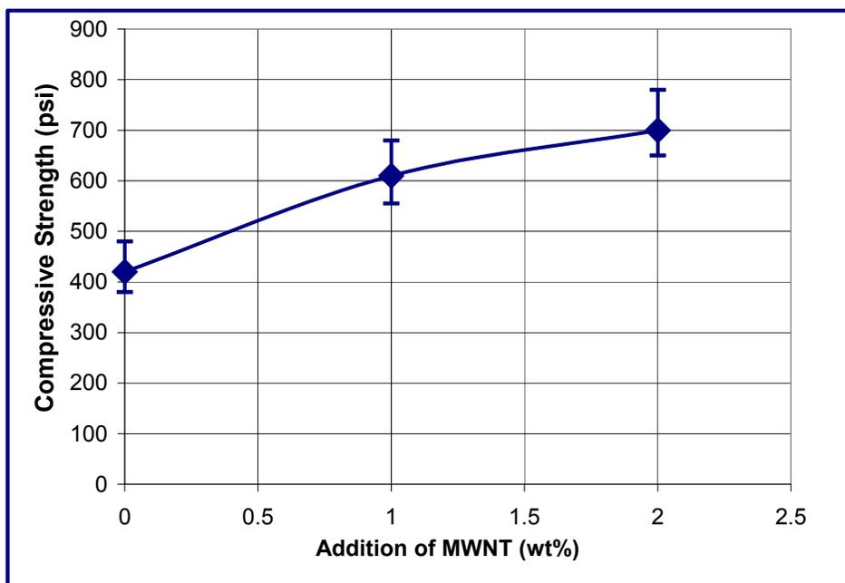
Figure 3. Effect of Nanotube Infiltration on Strength.
