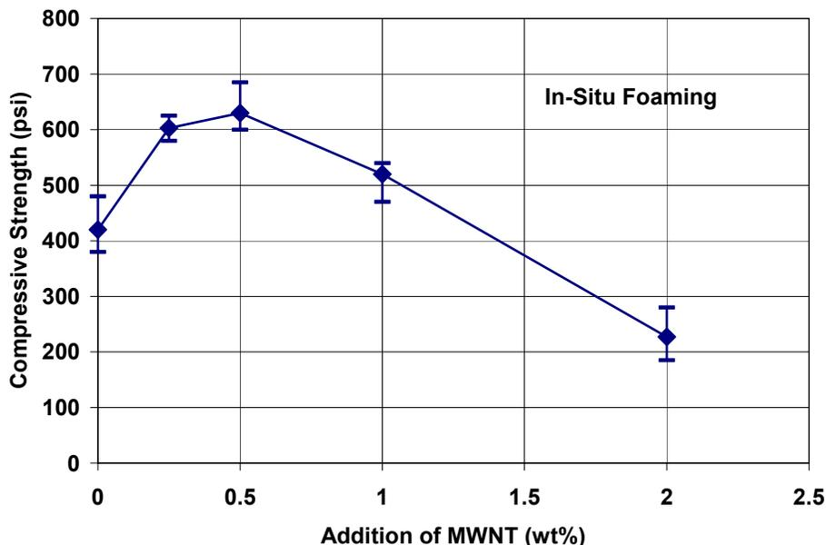
Figure 1. Effect of Nanotube Addition on Compressive Strength of High Thermal Conductivity Foam.
