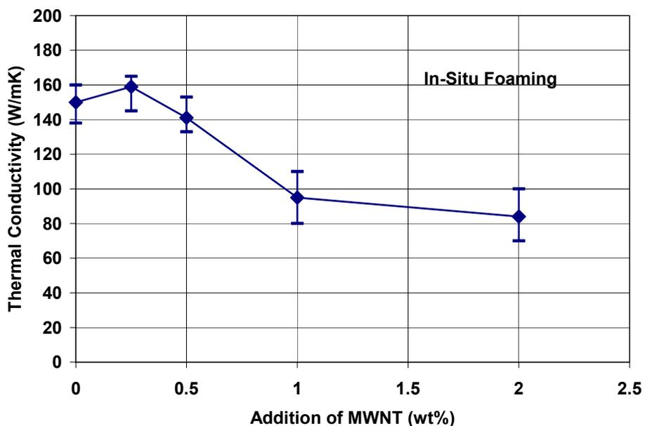
Figure 2. Effect of Nanotube Addition on the Thermal Conductivity of High Thermal Conductivity Foam.
